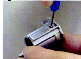
Pin gauge to measure hole dia.
