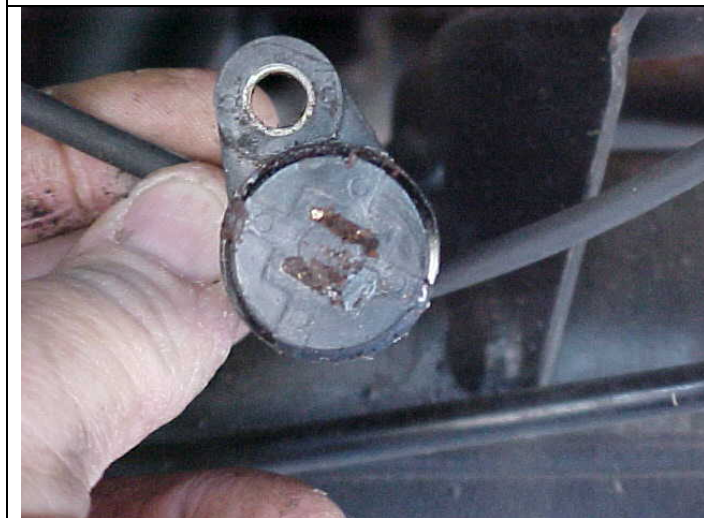
Debris found on left rear wheel speed sensor
