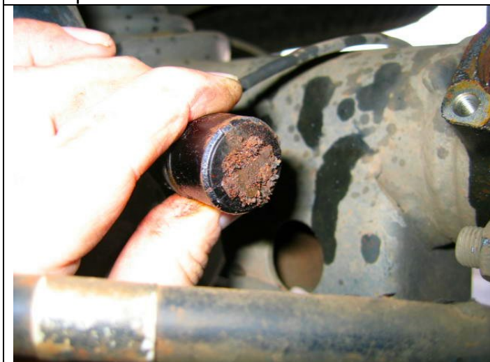
Contamination on speed sensor.
