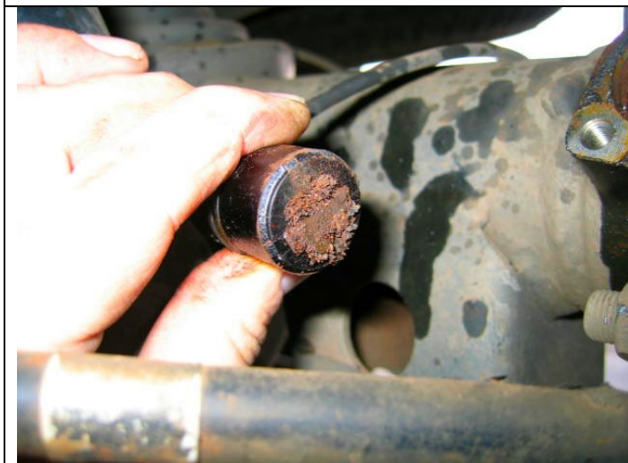
Debris on rear ABS wheel speed sensor
