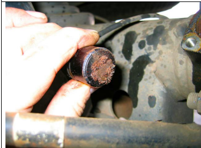
Debris on rear ABS wheel speed sensor
