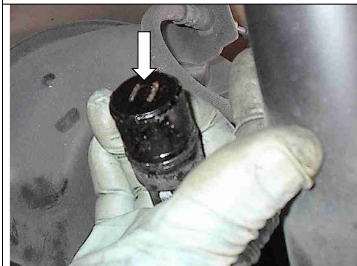
Debris/Rust on the right rear ABS wheel speed sensor.
