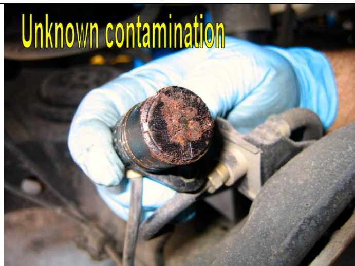
Contaminated speed sensor
