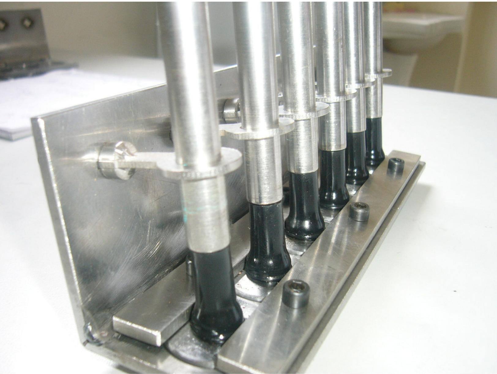
Shanghai Baolong Industries Co - We Recieved Some Valve Stems That Are Old Parts Diffrent Part Numbers On The Box. Not Enough Grease Or Lubricate On Them Causing Then To Split And Break Apart Parts Are In Iq Awaiting Supplier Review.
