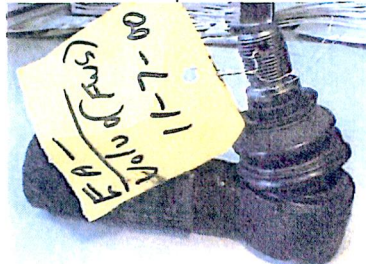
Foto 2: press-in side with disassembled sealing
