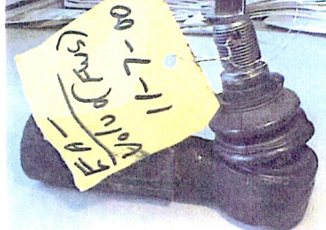
Foto 2: press-in side with disassembled sealing
