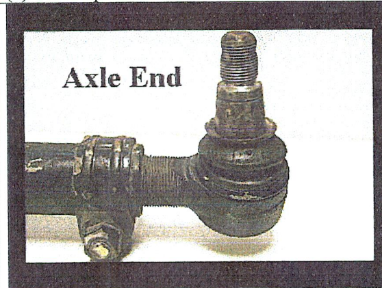
(e) Axle end of 102,700 mile drag link
