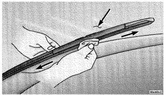
Use a sponge or soft cloth and a mild non abrasive cleaner to remove accumulations of salt and/or road film from the rubber edges of the blade. Consult the maintenance schedule for proper service intervals.
