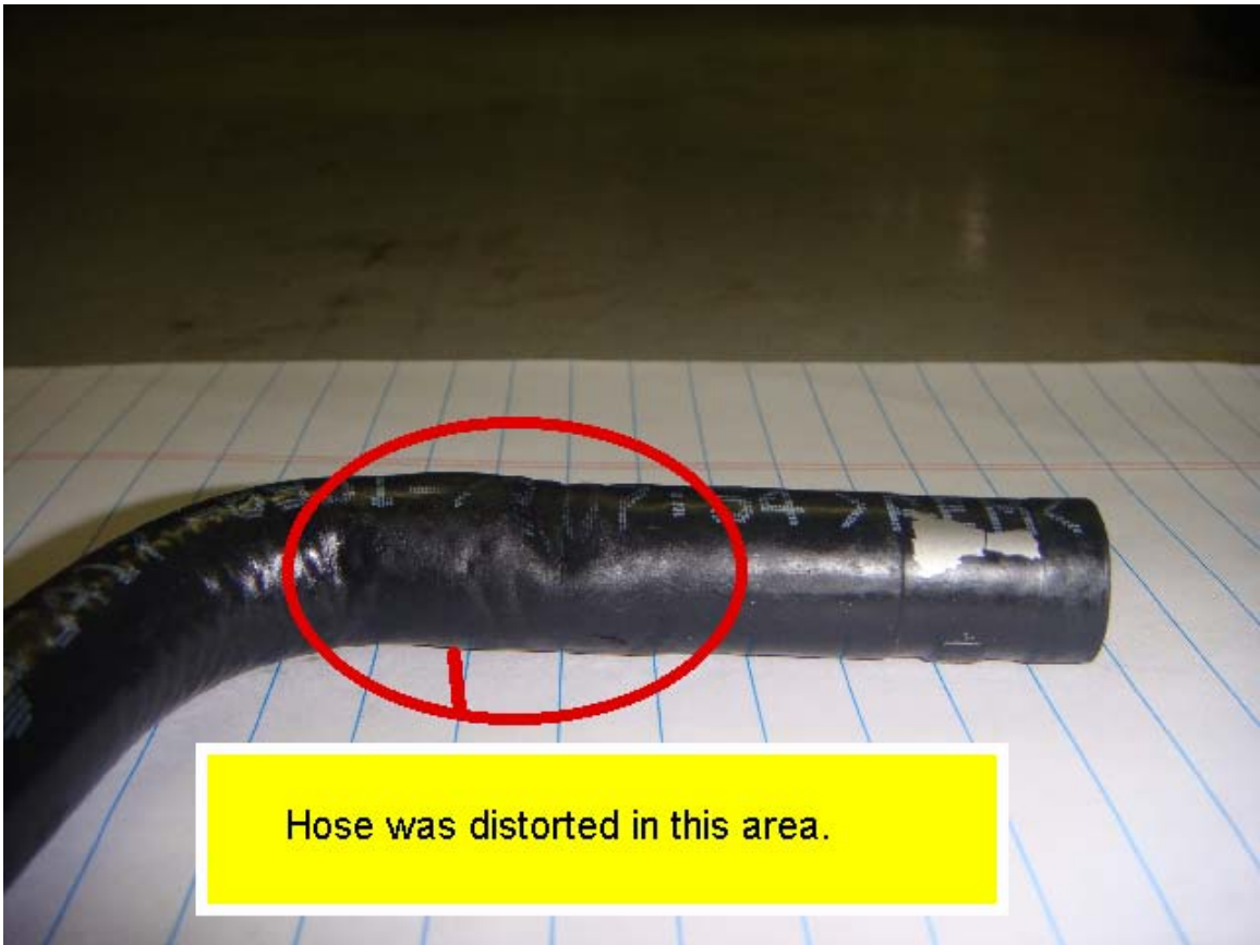
View of location of fluid leak at cooler hose
