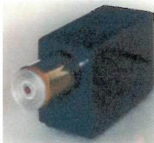
Innovation : 9000 RPM test rig for rotating telemetry power source used standard off the shelf components in a novel way
