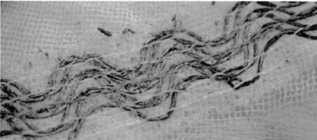
Middle - electrode of W211 from testreport 1632/1 page 24 - 28 after NOS-RUSH-TEST
