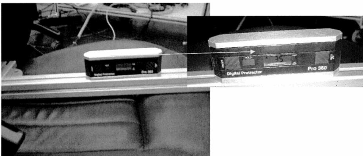
Image #7: angle of seat cushion (for mechanical durability test): 3.5°
