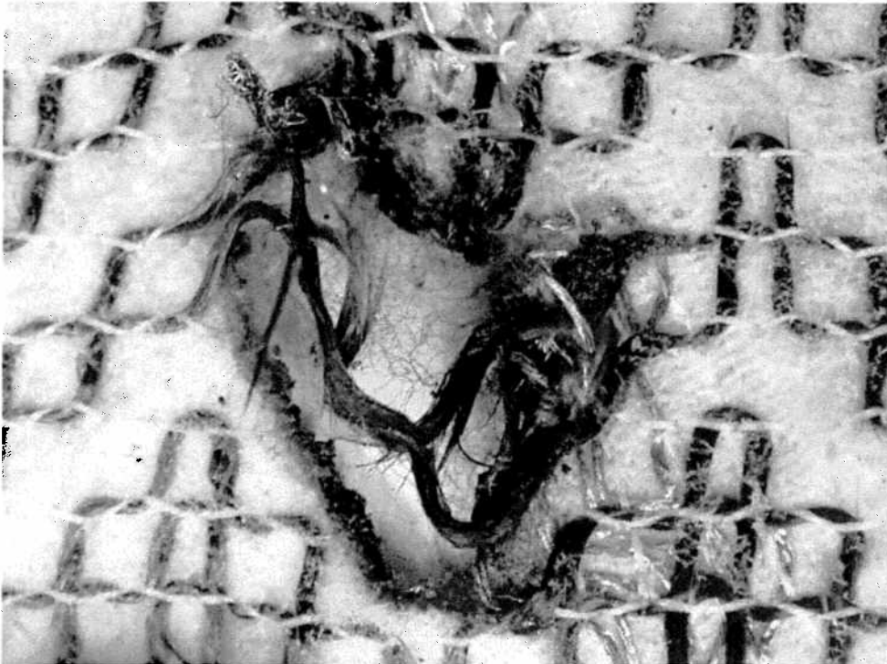
Fig 26: detail of the broken electrodes
