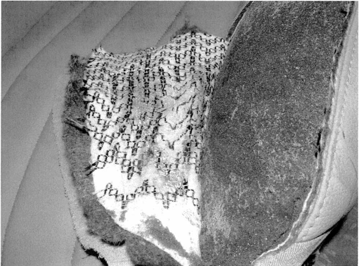
Image #6: rubbed off Carbotex fibres in the contact area of the test form.
