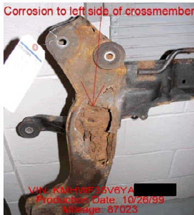
- Crossmember corrosion to both sides. VIN: KMHWF35V6YA [REDACTED]
