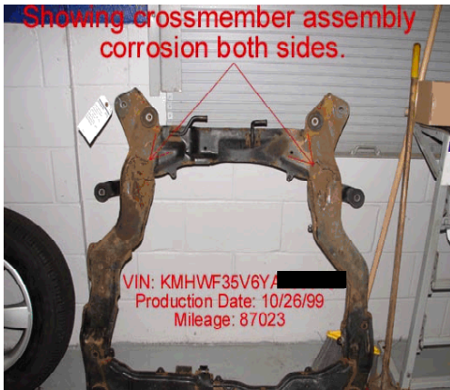
- Crossmember corrosion to both sides. VIN: KMHWF35V6YA [REDACTED]
