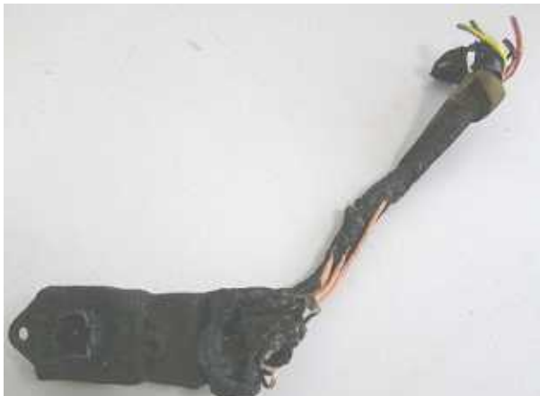
Carbonization of P/W SW case, insert-molded base, connector and harness.
