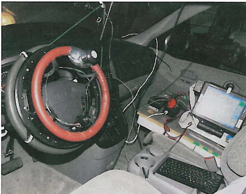
Figure 8 - Data Acquisition System Installed in Kia Sedona
