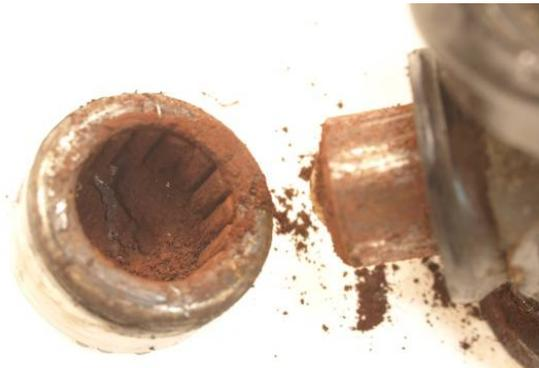
Figure 3. Corroded SIS universal bearing.
