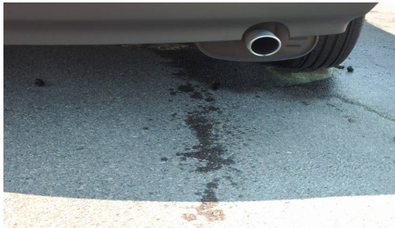
Figure 1: Example of a power steering fluid leak
