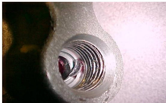
Figure 2: Damaged threads in the tube nut
