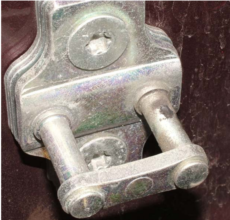
Striker on Body at Rear of Left PSD
