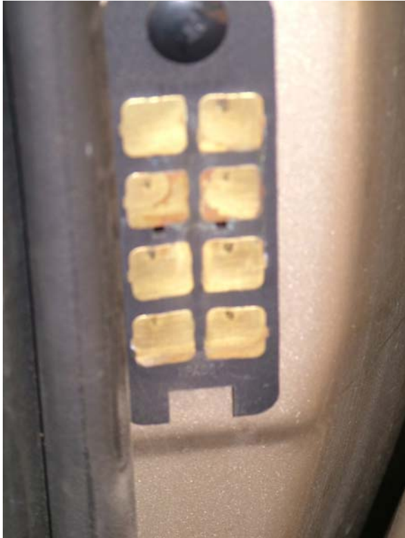
Electrical Contacts on B-Pillar for Right PSD
