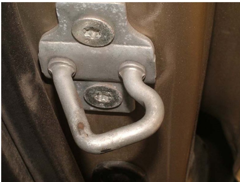
Striker on Body at Front of Right PSD
