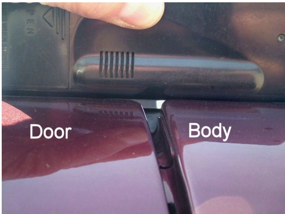
Proper Vertical Alignment of Top Rear of Left PSD with Roof
