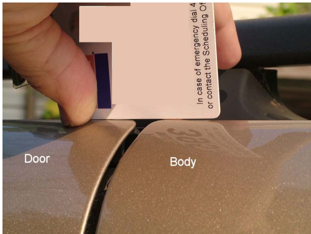
Proper Vertical Alignment Top Rear of Left PSD with Roof
