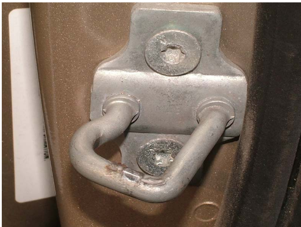
Striker on Body at Front of Left PSD
