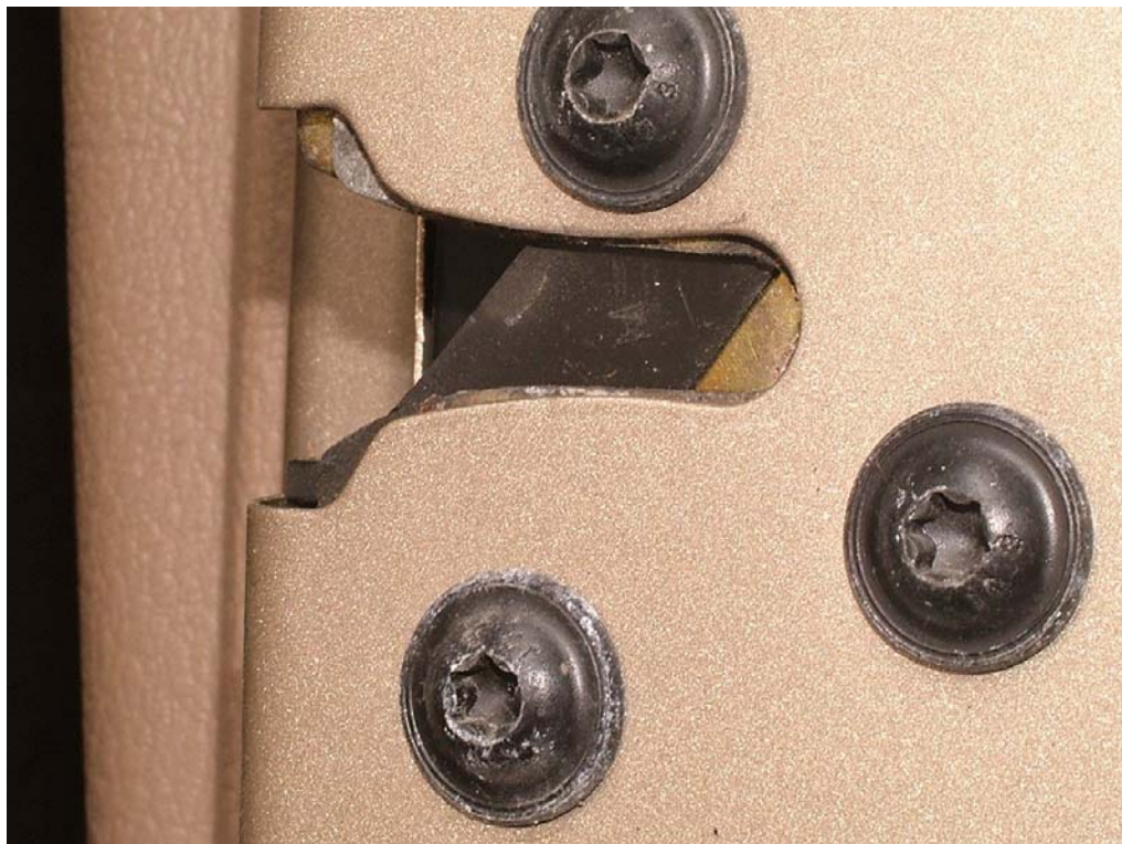
Latch Mechanism at Front of Right PSD
