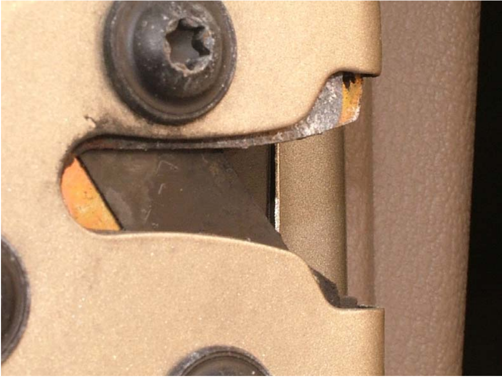
Latch Mechanism at Front of Left PSD
