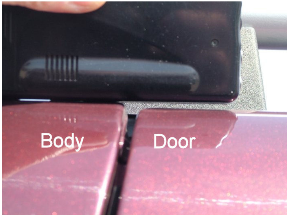
Vertical Misalignment of Top Rear of Right PSD with Roof
