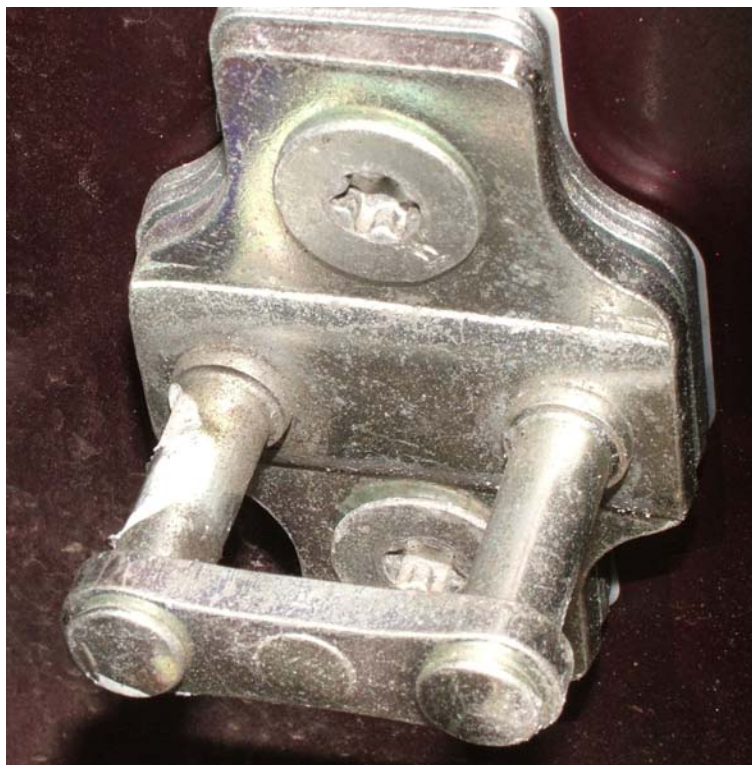
Striker on Body at Rear of Right PSD
