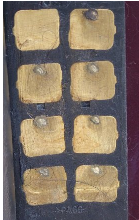
Electrical Contact Pads on Right PSD
