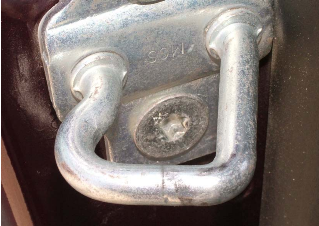
Striker on Body at Front of Left PSD
