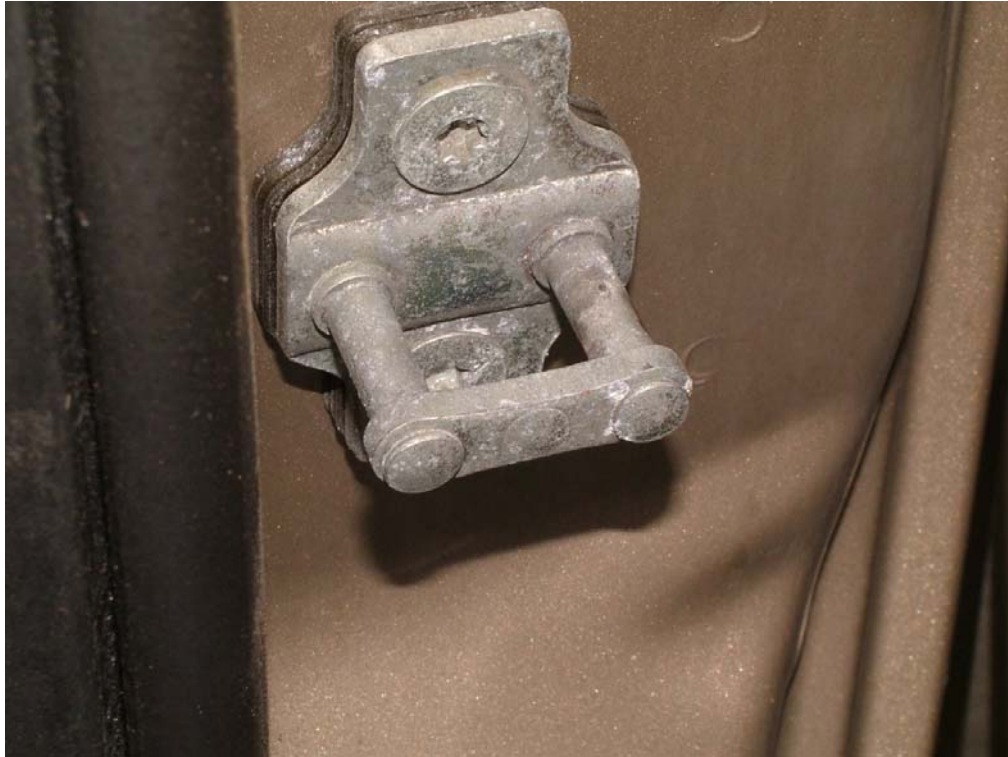
Striker on Body at Rear of Left PSD
