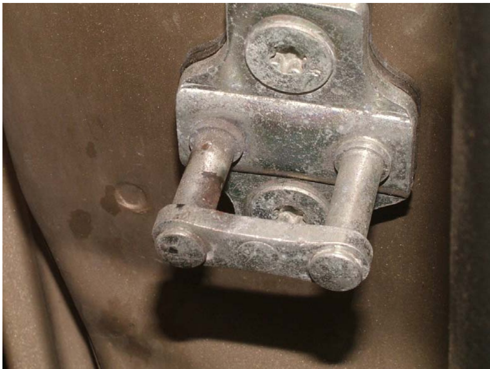
Striker on Body at Rear of Right PSD
