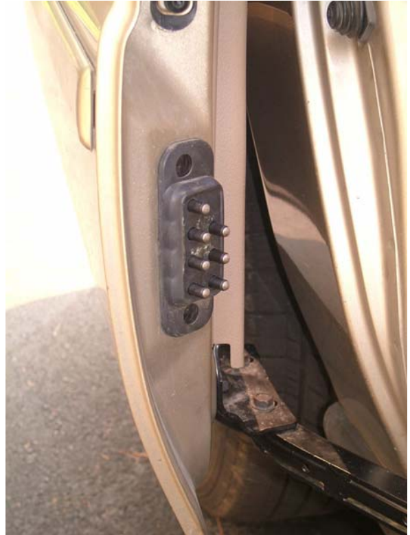
Electrical Contacts on Front of Right PSD
