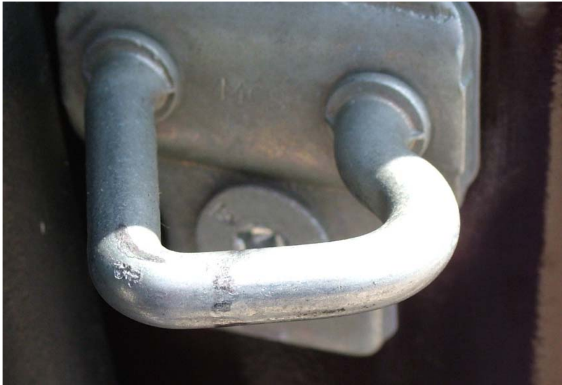
Striker on Body at Front of Right PSD
