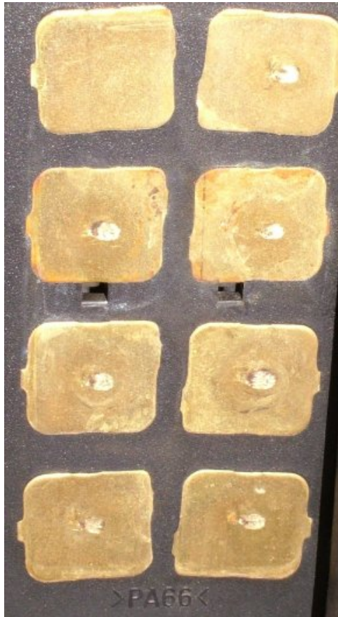
Electrical Contact Pads on Left PSD
