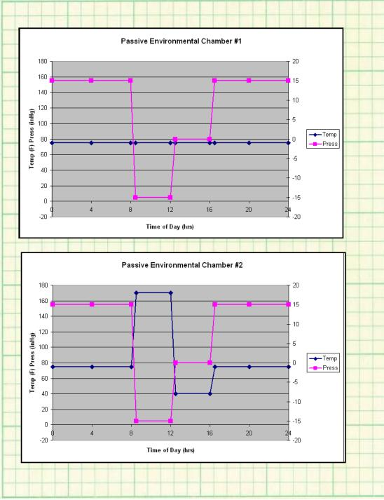
These chambers were always humid and had the same pressure/vacuum changes. Chamber #2 also under went 4 hours in the oven and 4 hours in the refrigerator. Changes in an environmental chamber are usually automated, but these chambers required manual attention three times a day, so they were called "passive chambers".
