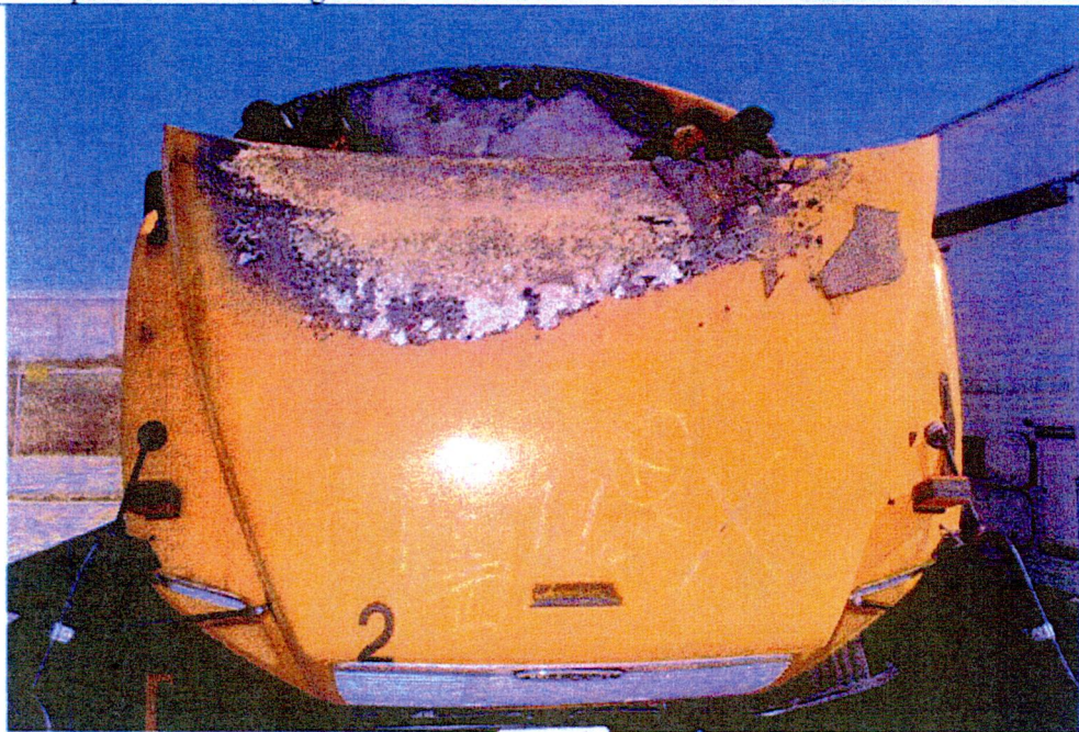
This photo shows burn damage to top of engine hood.
