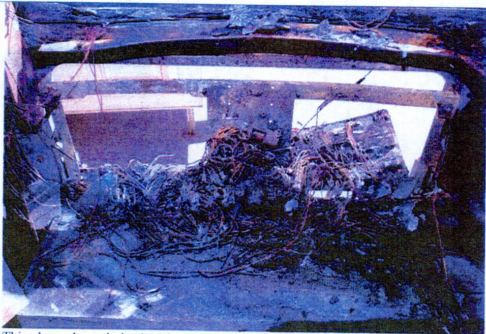
This photo shows holes in driver's side of bus due to broken windows.
