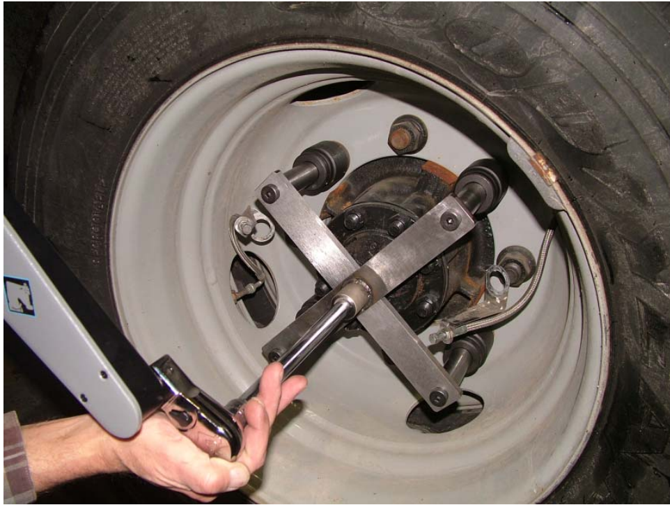
Figure 5 - The Wheel Torque Crossbar and Beam-Type Torque Wrench in Use at a Rear Wheel
