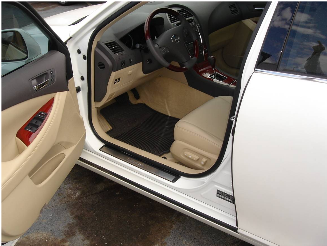
Photo 2: Driver floor mat, as found at start of inspection process
