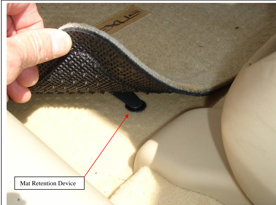
Photo 5: Driver floor mat, as found at start of inspection process
