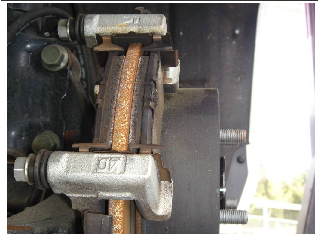
Photo 7: RHR rotor and pads, caliper removed
