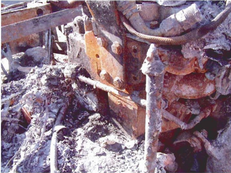
Figure 13 – Front of Engine After Large Debris Had Been Removed and Small Debris Sifted and Removed
