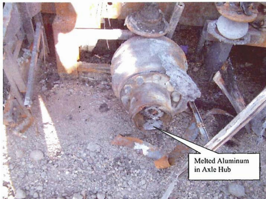
Figure 6 – Melted Aluminum from the Wheel was Found in the Right Rear Axle Hub of the Motorhome
