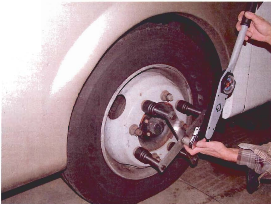
Figure 4 - The Wheel Torque Crossbar and Beam-Type Torque Wrench in Use at a Front Wheel
