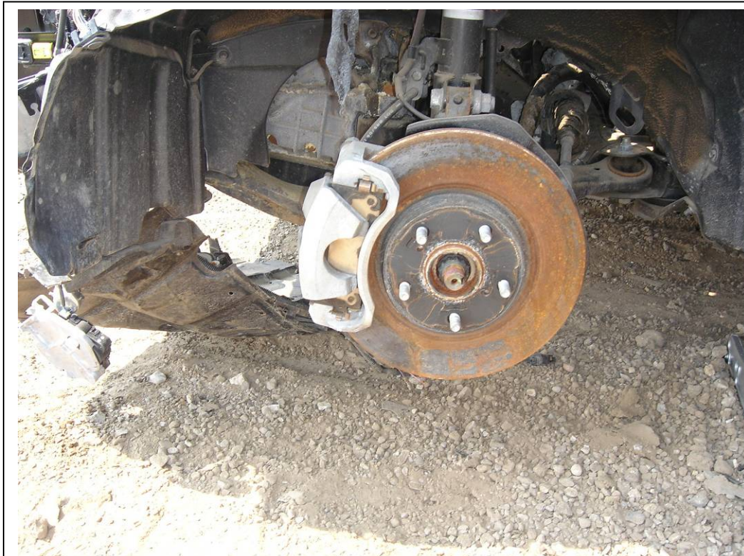
Photo 7: LHF brake assembly, wheel removed
