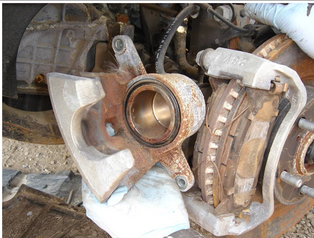
Photo 8: LHF brake hardware, caliper removed
