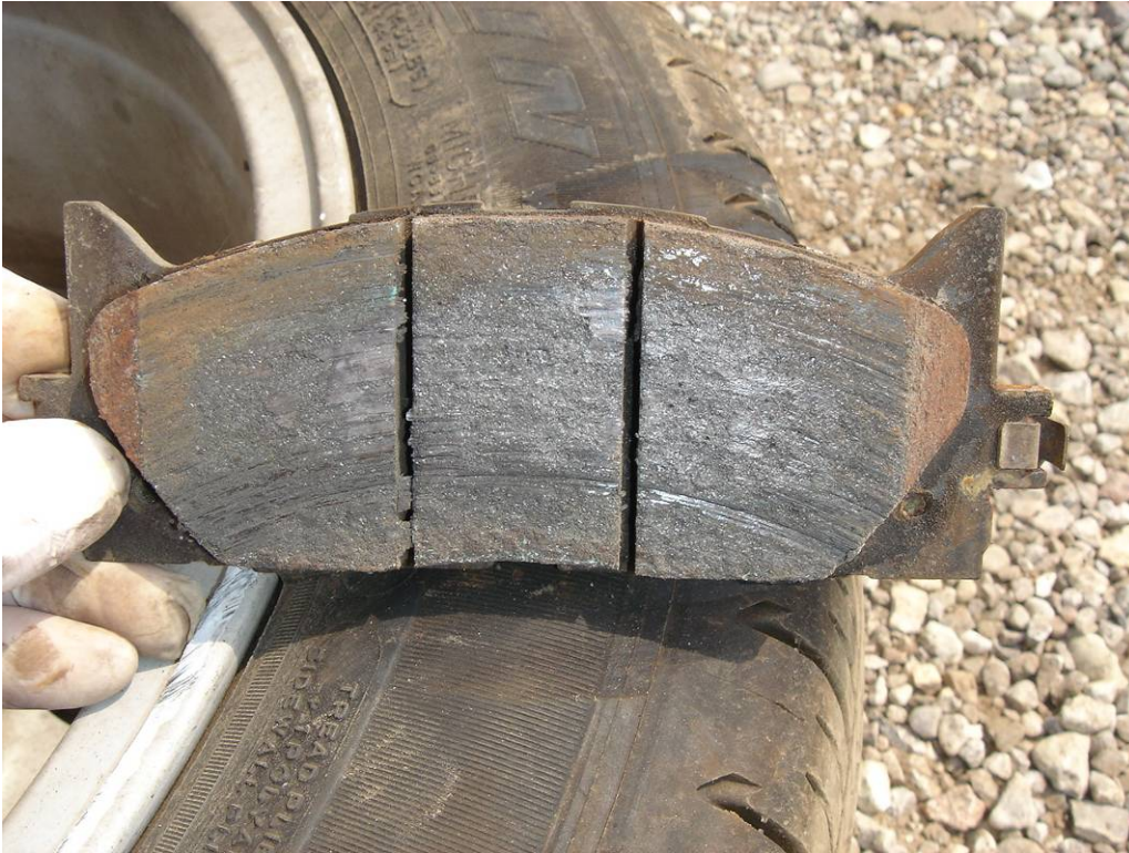
Photo 9: LHF disc brake pad, friction surface/rotor side
