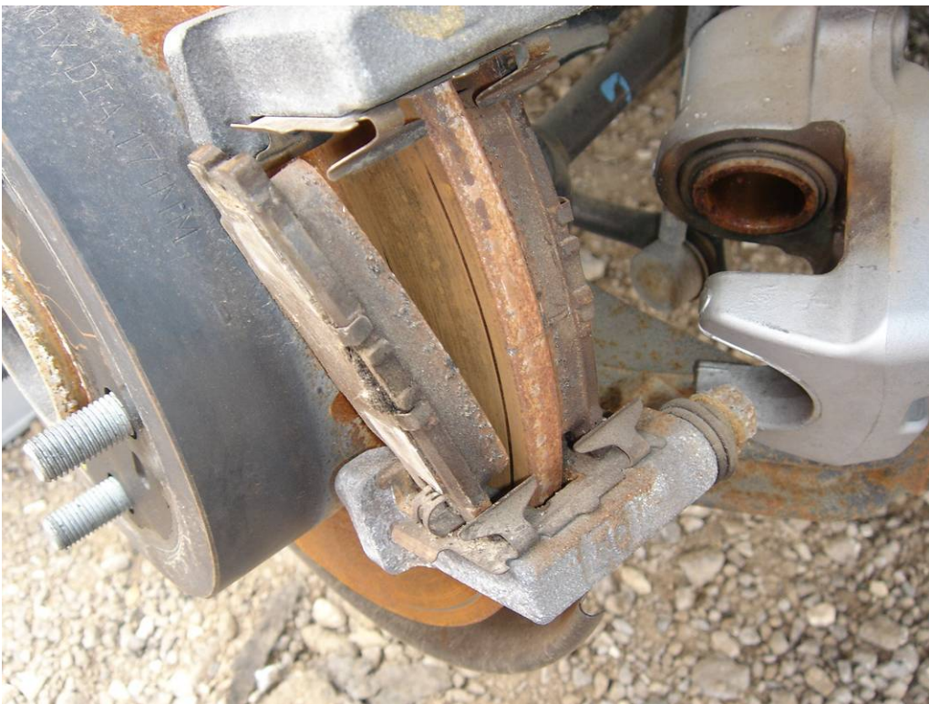
Photo 10: LHR disc brake hardware, caliper removed
