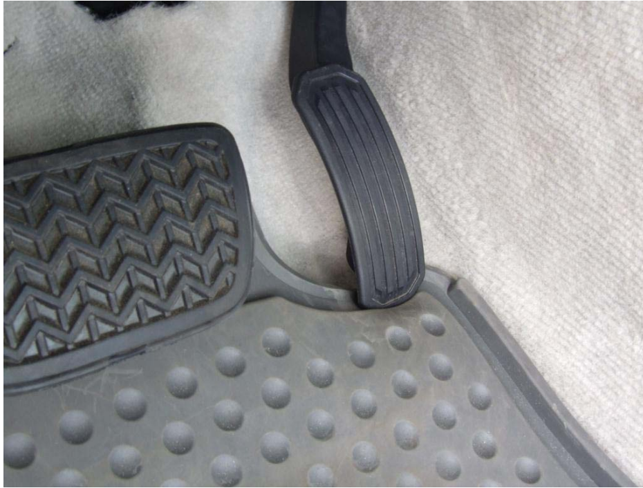
Figure 3 – Accelerator Pedal Trapped at Full Throttle by Unsecured Rubber Floor Mat
