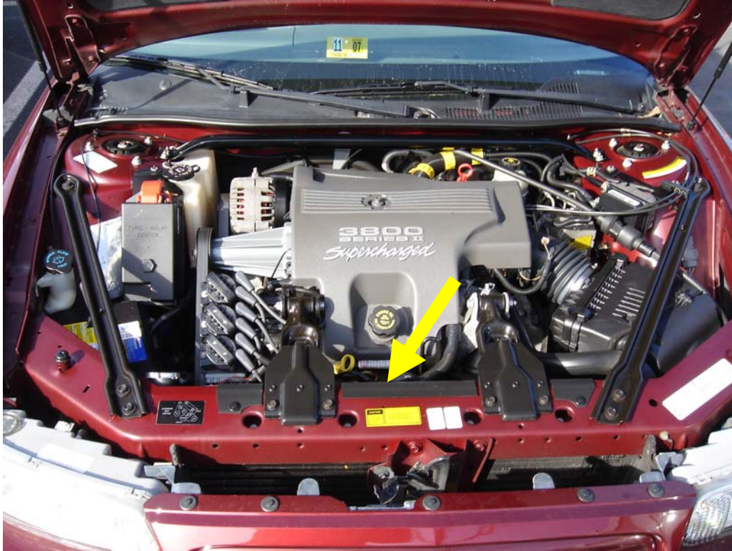
Figure 1: Exemplar Vehicle (yellow arrow shows subject fire area of origin)
