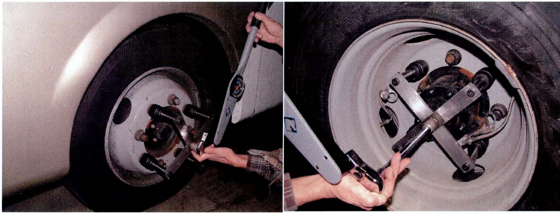
Figure 4 - Wheel Torque Crossbar and Beam-Type Torque Wrench to Measure Normal and Abnormal Drag on Rotating a Raised Wheel
