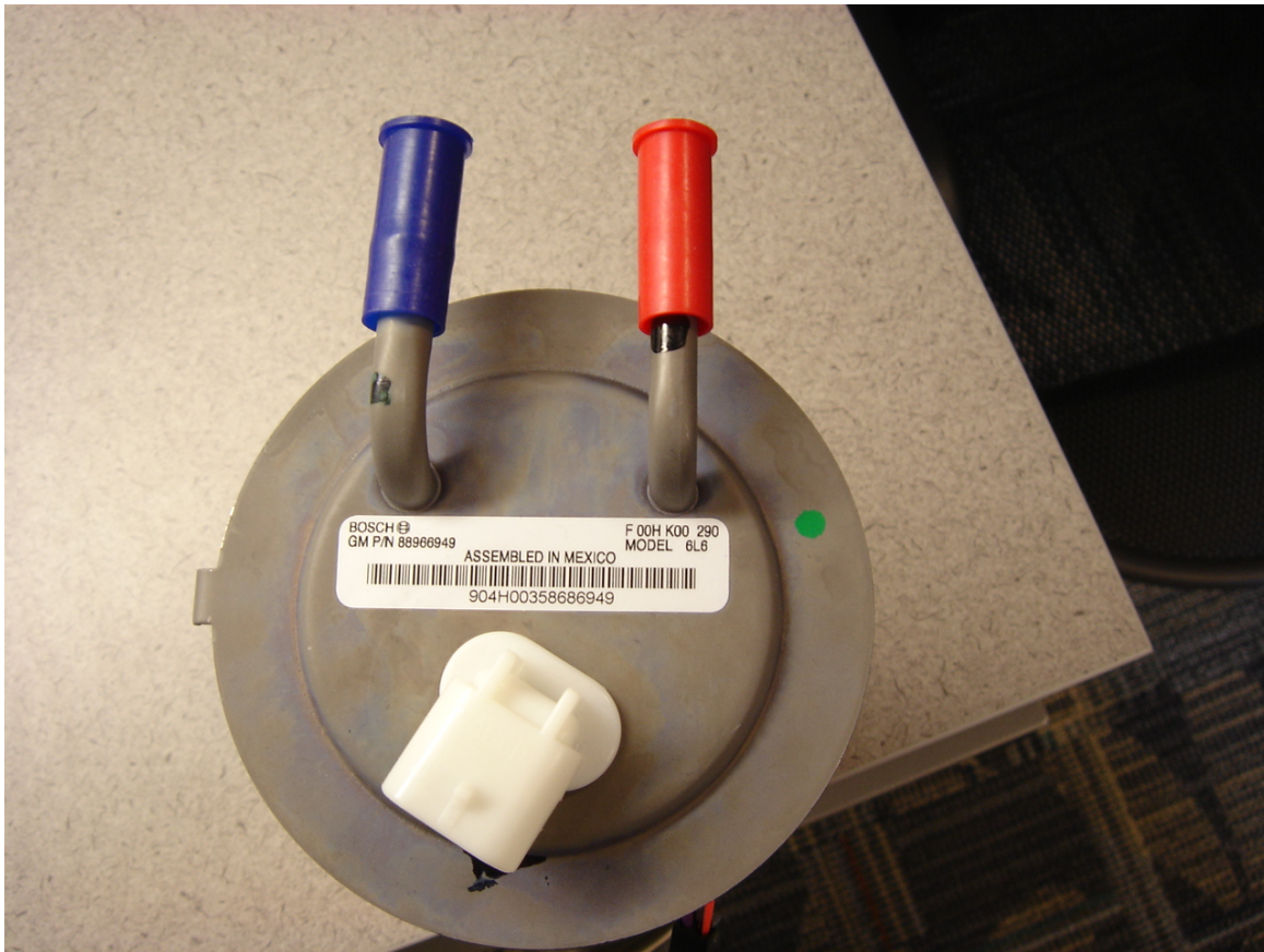
Figure 2: Metal Supply and Return Lines from top of MRA Flange
