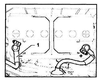
Disconnect negative (-) battery cable -1- from battery
