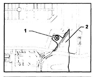
Remove bolt -1- from battery box cover and remove air duct -2-
