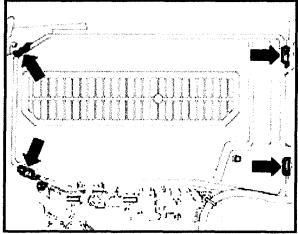
Open battery box clips -arrows- and remove cover
