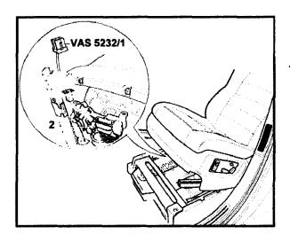
Insert airbag adapter VAS 5232/1 into connector socket -2- of passenger's or driver's seat
