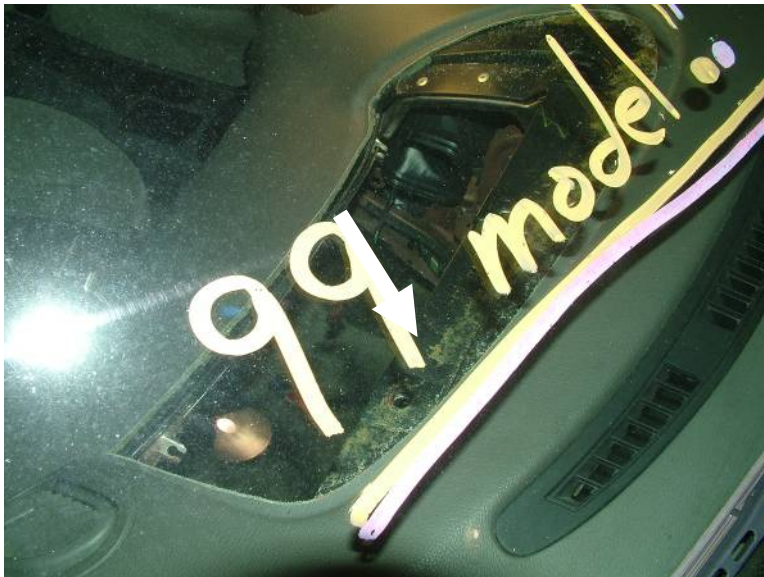
1999 Contour non-complaint vehicle showing position of defroster register with respect to SRS location. Figure 47 – SRS Inspection Showing Register In instrument panel
