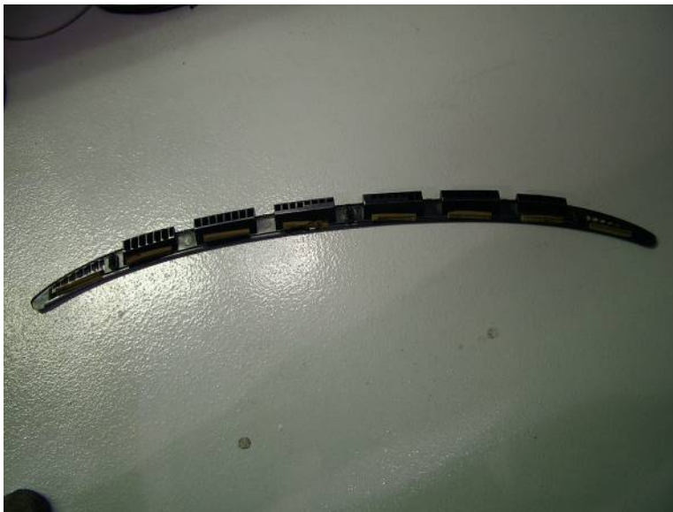
1999 Contour non-complaint vehicle defroster register underside after removal from the vehicle. Figure 49 – SRS Inspection, Bottom View of Register
