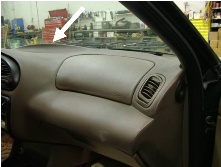
Figure 6 – 2000 Ford Contour with Warped Instrument Panel (Hillsdale MI)
