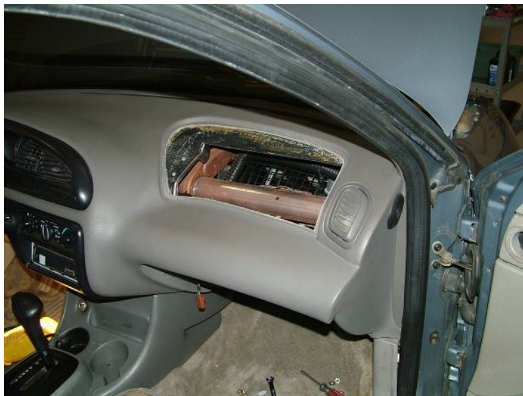
Figure 40 – SRS Inspection, Cover Removed
