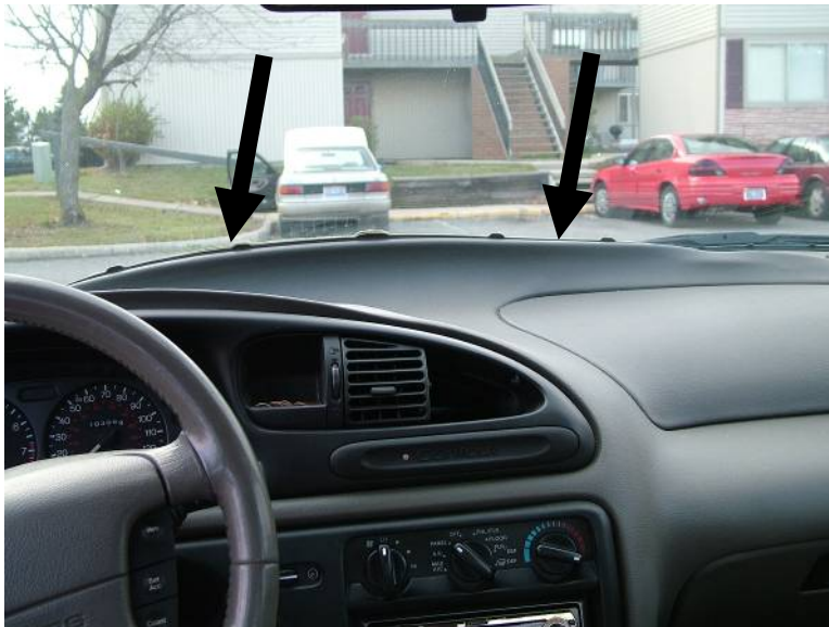
Arrows show instrument panel warpage on driver's and passenger's sides of the vehicle. Figure 9 – 2000 Ford Contour with Warped Instrument Panel Close-up (Lima OH)
