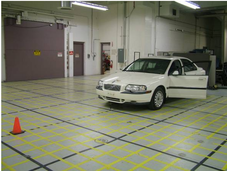
1999 Volvo S80 peer vehicle positioned on sight distance grid in preparation for testing.
