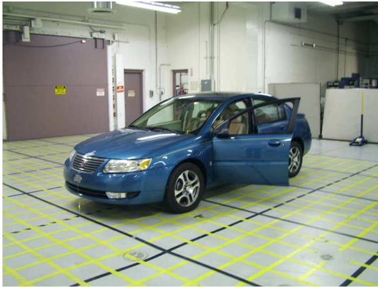
2005 Saturn Ion peer vehicle positioned on sight distance grid in preparation for testing.
