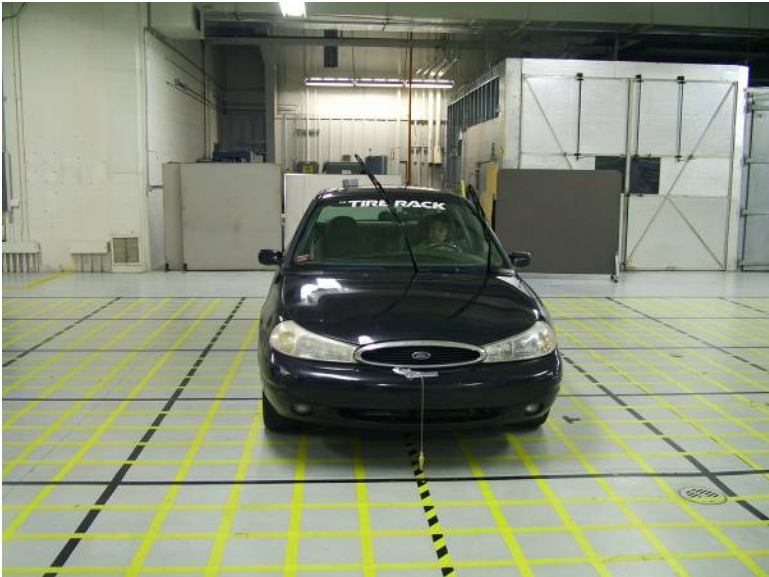
2000 Ford Contour complaint vehicle located on test grid. Note vehicle track width is within +3 ft and -3 ft. Figure 3 – 2000 Ford Contour – Warped Instrument Panel Forward Visibility Test
