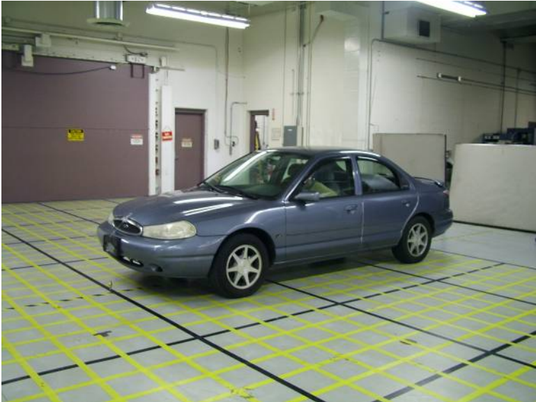
1999 Ford Contour non-complaint vehicle (good instrument panel) positioned on sight distance grid in preparation for testing. Figure 2 – 1999 Ford Contour Forward Visibility Test
