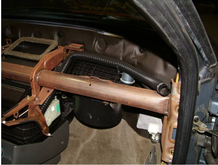
1999 Contour non-complaint vehicle with good instrument panel, with entire instrument panel assembly removed. Figure 46 – SRS Inspection View of Frame with instrument panel Removed.
