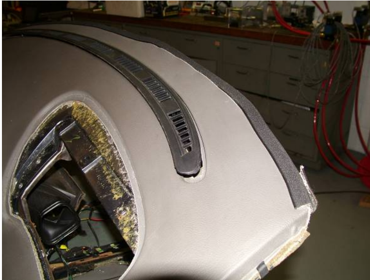
1999 Contour non-complaint vehicle instrument panel with register after removal from vehicle. Register was set in place. Figure 48 – SRS Inspection Showing Register In instrument panel, View 2
