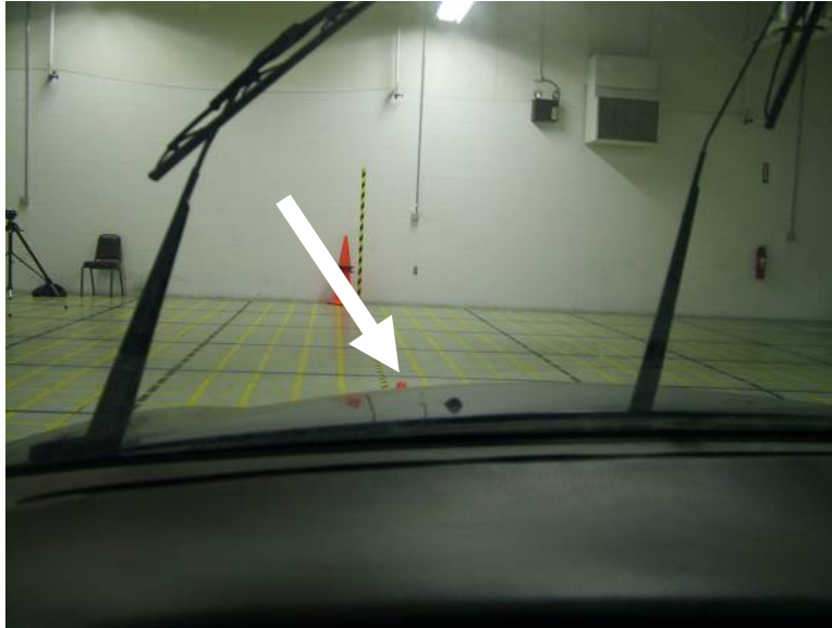
Figure 14 – Visibility Test - Cone Entering Field of View
