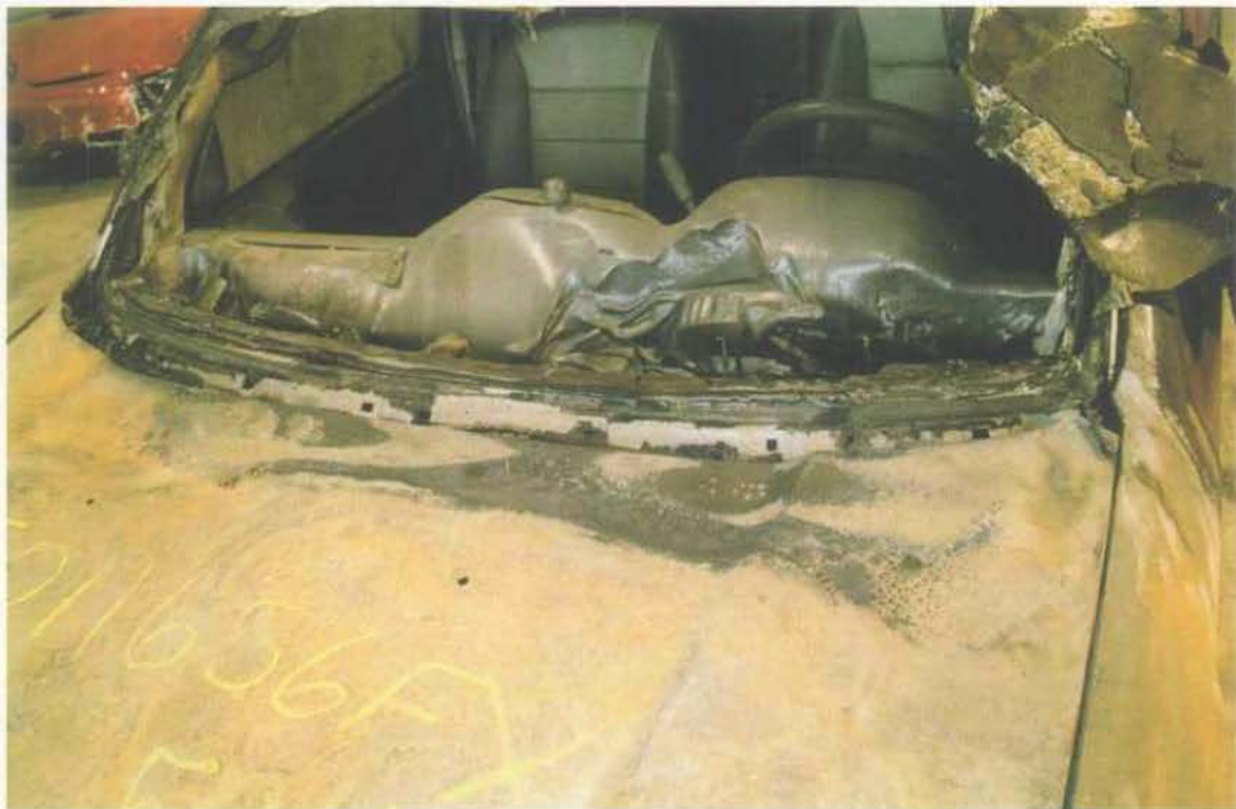
Photo No. 4: The burn patterns on the driver's side hood and dashboard.
