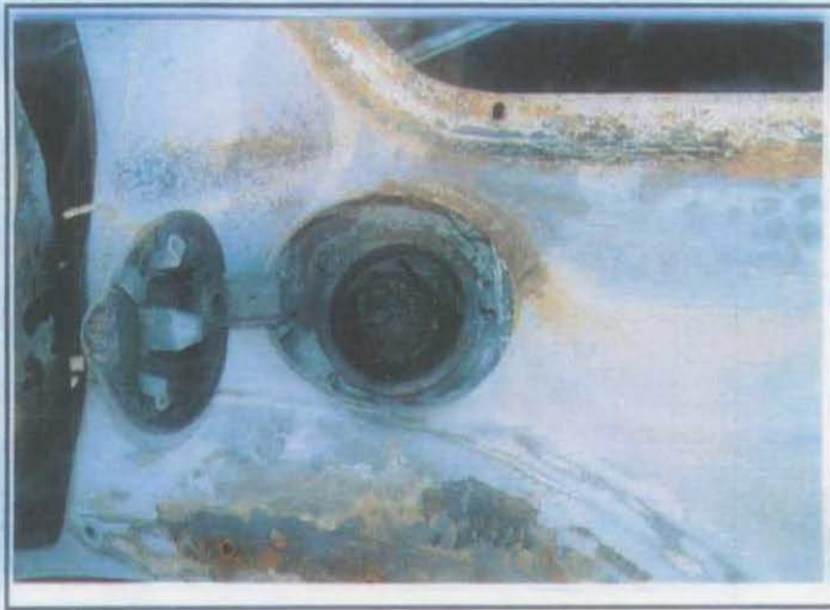
Figure 15. View of Melted Fuel Filler Neck Cap
