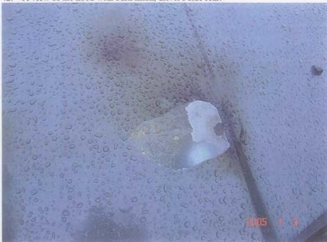
42. A view of the hood with burn mark, driver's side rear.
