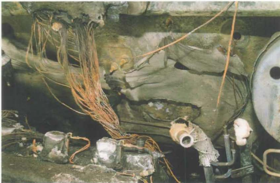
Photo No. 42: Overall view of the rear wire harness next to the master cylinder.
