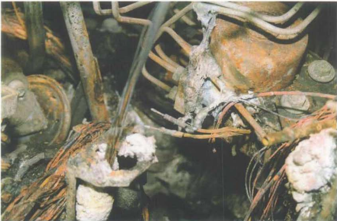
Photo No. 40: Overall view of the wire harness directly below the master cylinder.
