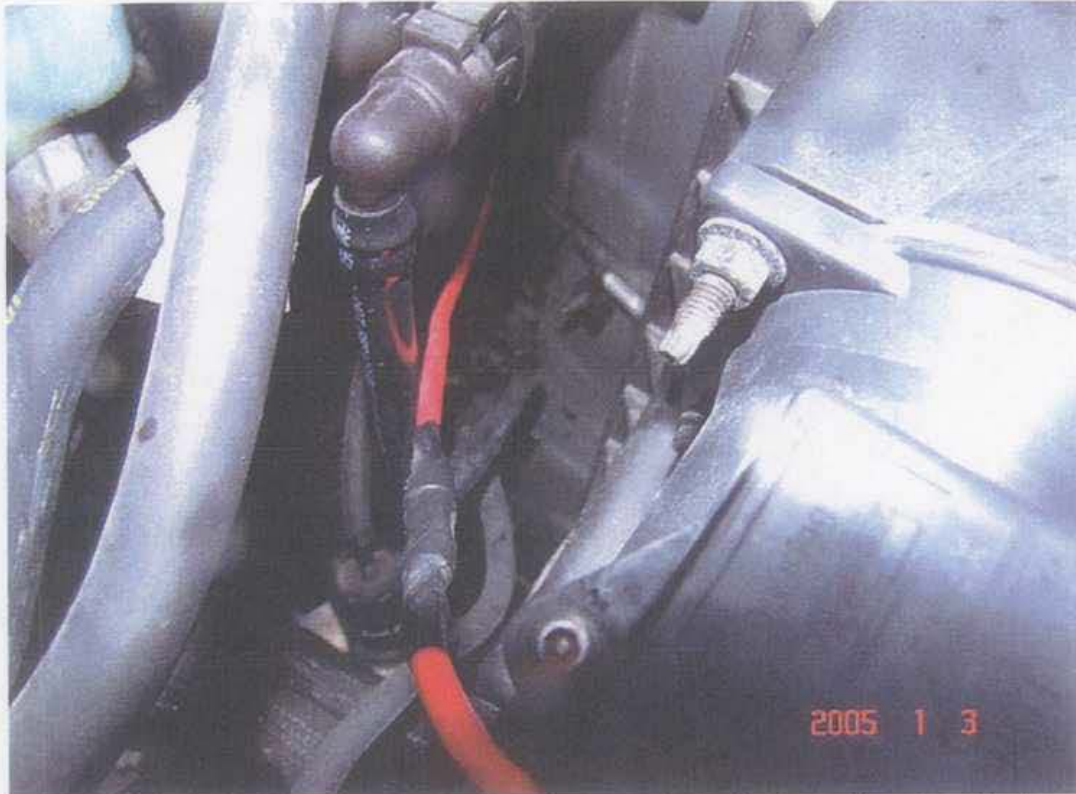
27. A view of the aftermarket wiring heading towards the brake wall on the driver's side.
