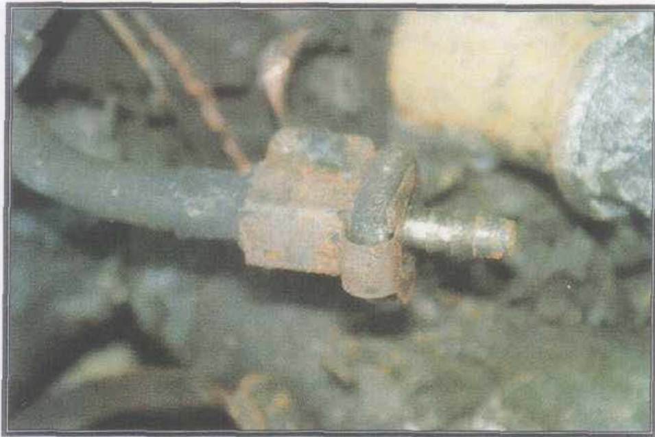
Photograph 13 (Closer view of flexible fuel line connection point on engine side)
