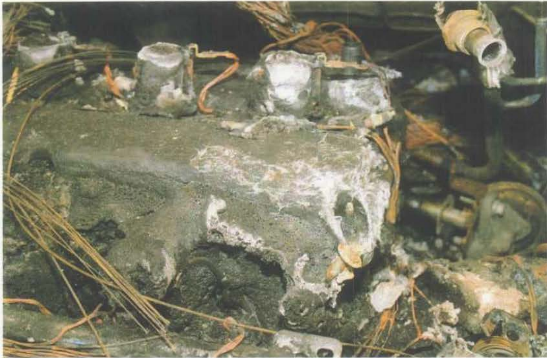
Photo No. 43: Directional burns on the engine block.
