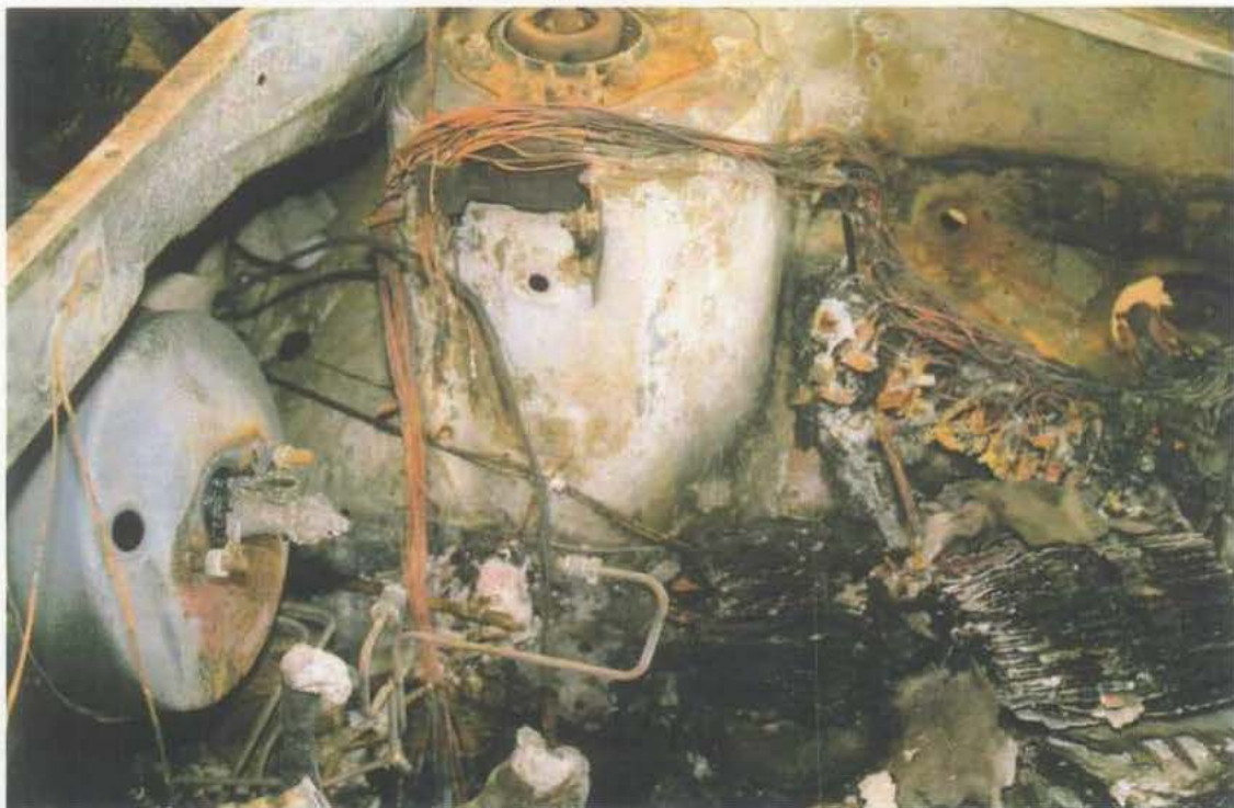
Photo No. 36: The directional burns on the driver's side of proportion of the engine compartment.
