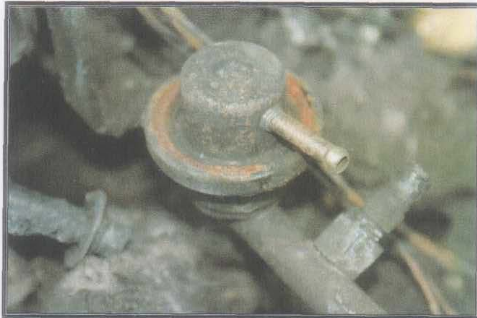
Photograph 14 (Fuel pressure regulator)
