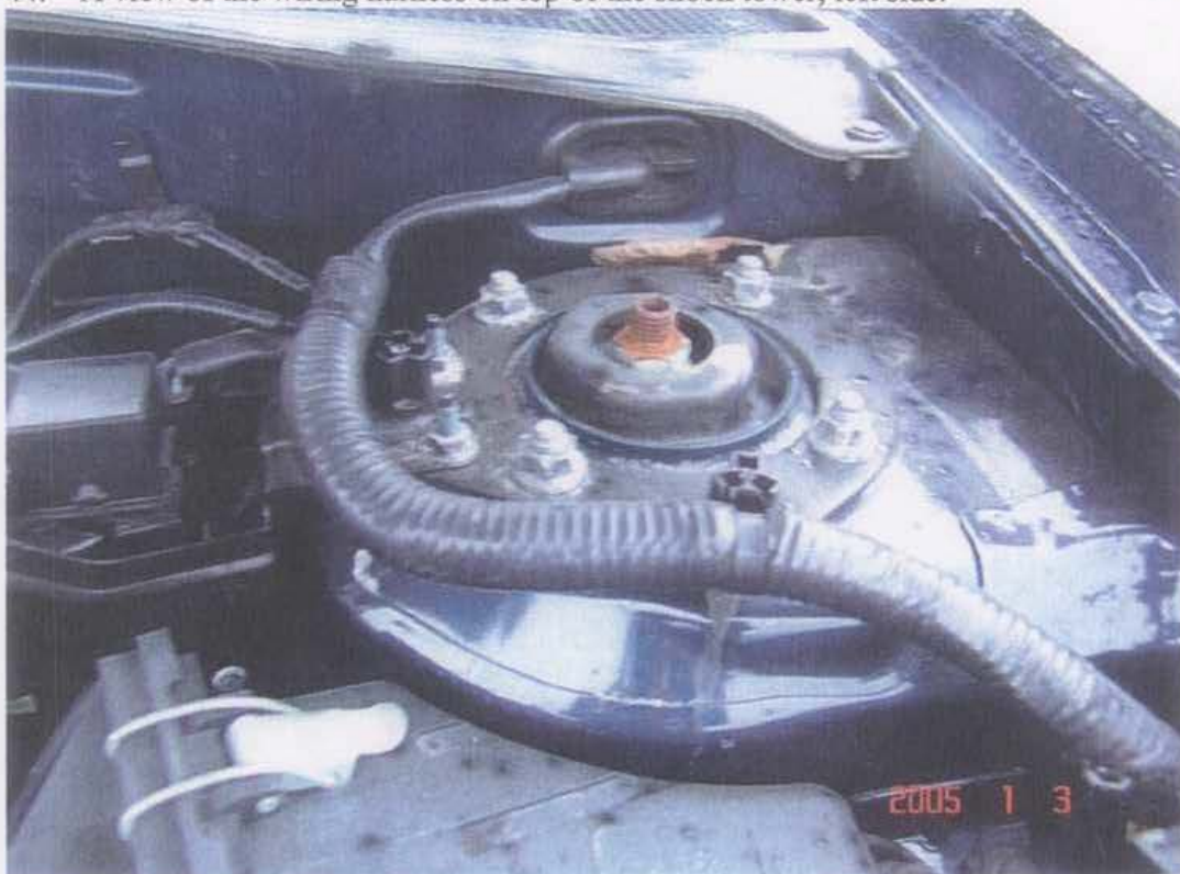
44. A view of the wiring harness on top of the shock tower, left side.
