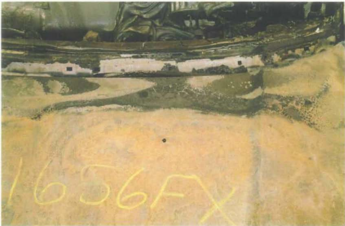
Photo No. 8: The burned area on the driver's side rear portion of the hood.
