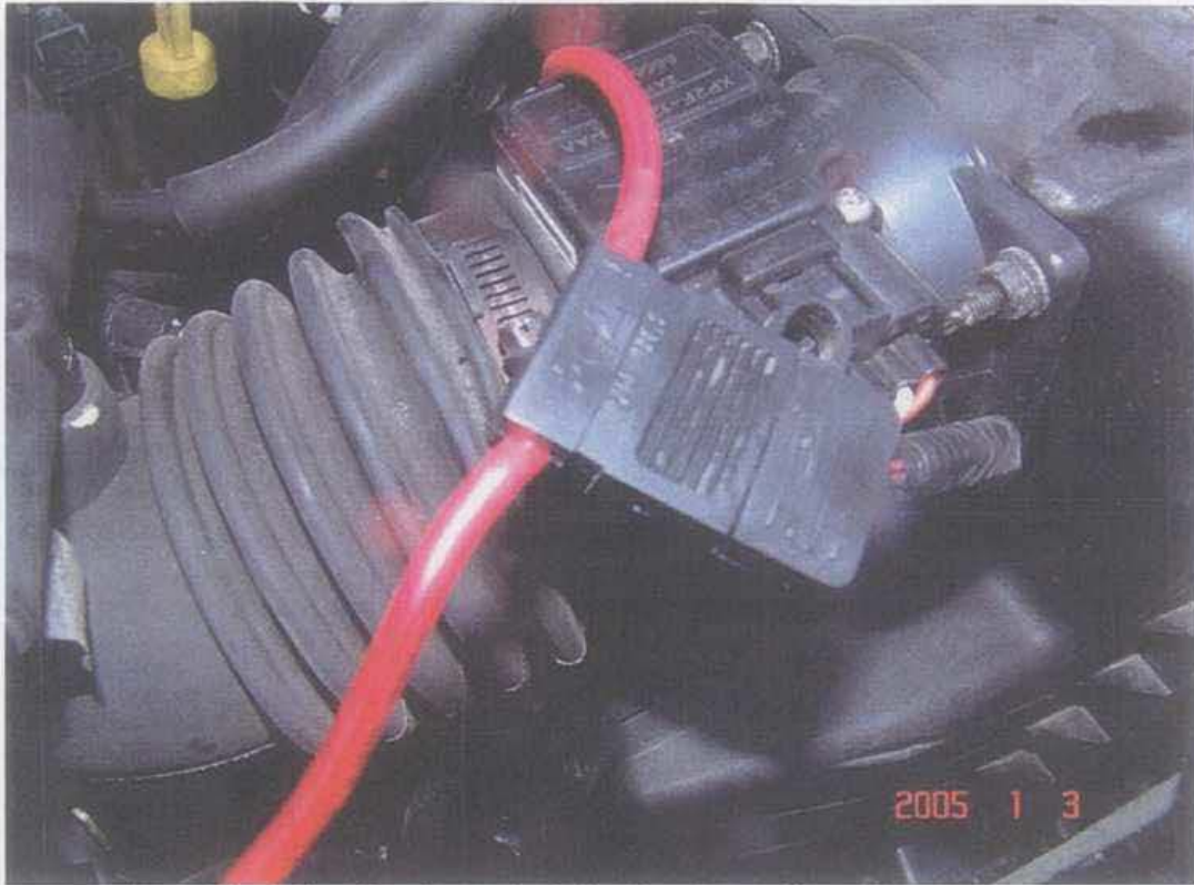
25. A view of the inline fuse located within the aftermarket wiring.
