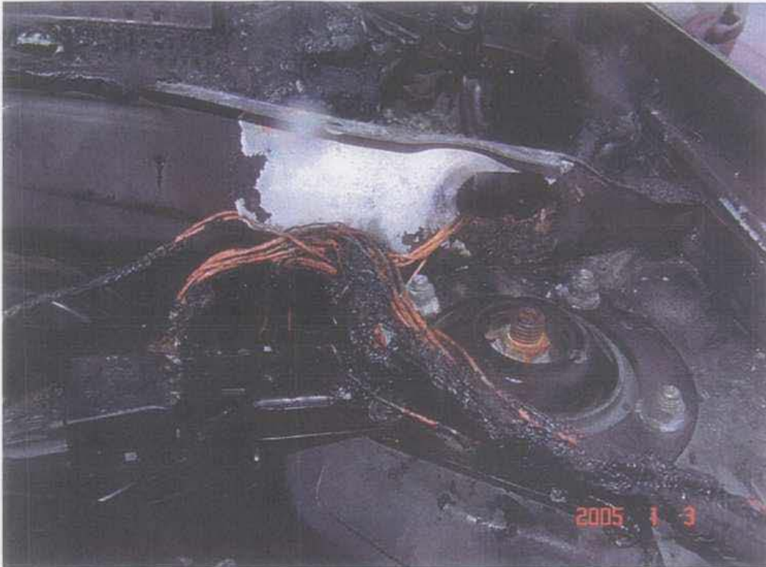
33. A view of the electrical wiring factory harness top of the shock tower, driver's side of the engine compartment.
