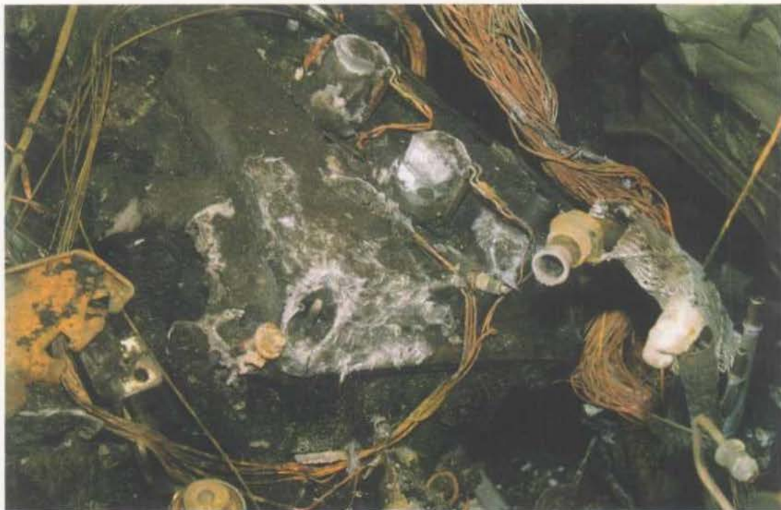
Photo No. 34: Directional burn patterns on the driver's side of the engine block.
