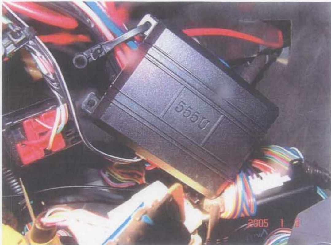
35. A view of the aftermarket remote start unit marked 555U.
