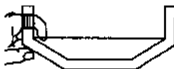
Improper Oil Level
