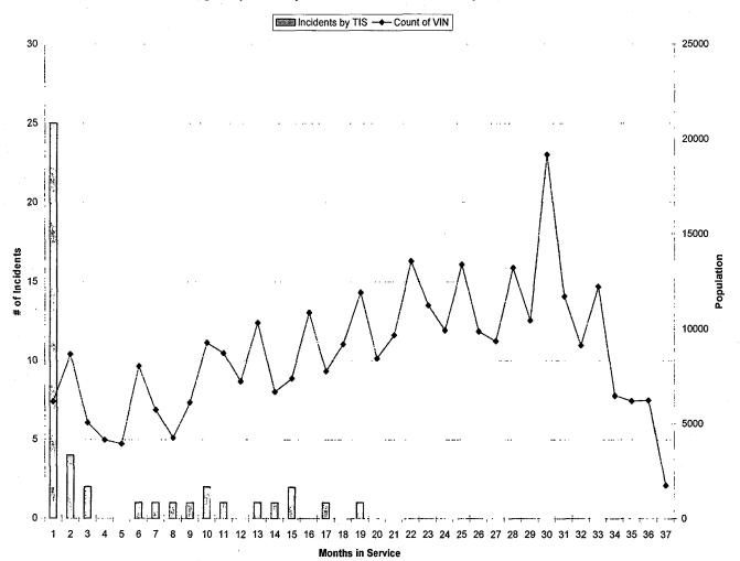
ODI analyzed the data to determine the likelihood of future failures in MY 2004 through 2006 Dodge Durango vehicles. The failure rate for the Durango intermediate shaft coupling bolts being loose or missing is 3.5 per 100,000 units (9 field reports, 2 complaints to DCC and 1 complaint to NHTSA). The warranty claim rate is 0.01 percent (32 claims in 338,381 vehicles). Weibull analysis of this data indicates that the problem is an early life failure issue and further failures are unlikely.
