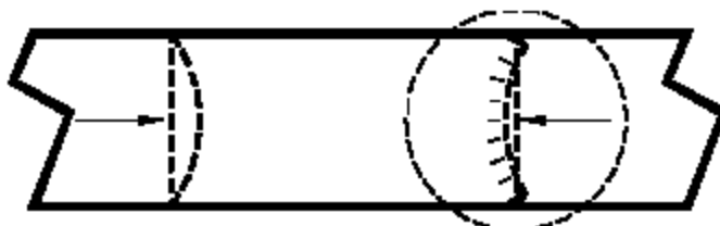
BULKHEADS DURING NORMAL OPERATION WITH HIGH VACUUM
