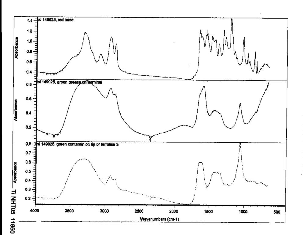
98-330: TSL # 149025: CONTAMINATION ON 77PS TERMINALS AT FORD/BOSCH
