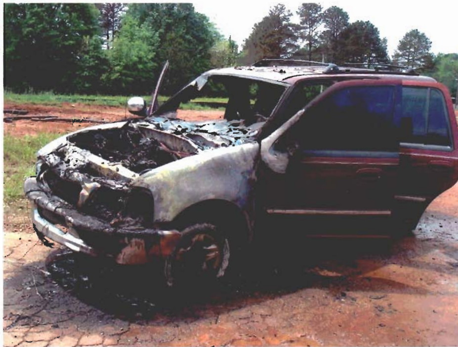
Figure 17. Burns Patterns On Test Vehicle.
