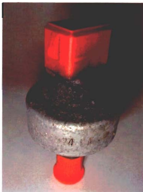
Figure 16. SCDS with melted base.
