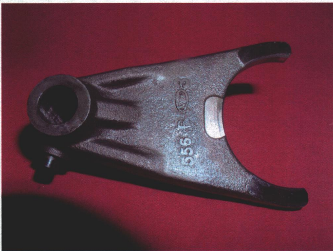
Figure 8 – Normal shift fork wear – 13,153 miles
