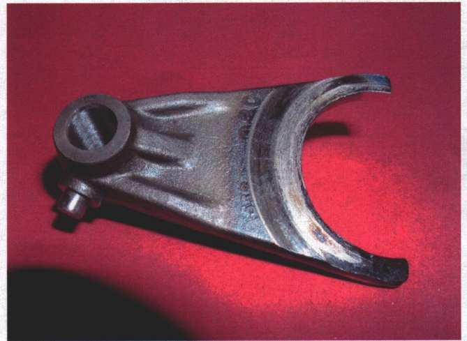
Figure 9 – Worn shift fork – 5,163 miles
