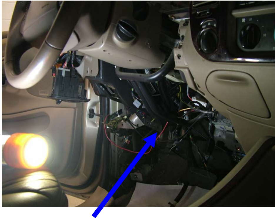
Figure 1: Location of the GEM and Fuse Box
