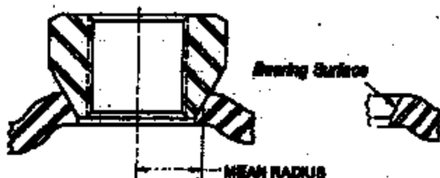
FIGURE 2—NUT SEAT BEARING SURFACE AND MEAN RADIUS
