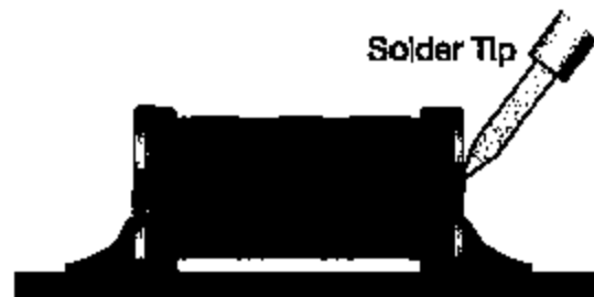
Poor Method - Direct Contact with Part
