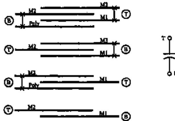
Figure 2.4-2 Various ways to implement capacitors using available interconnect layers. M1, M2, and M3 represent the first, second, and third metal layers respectively.
