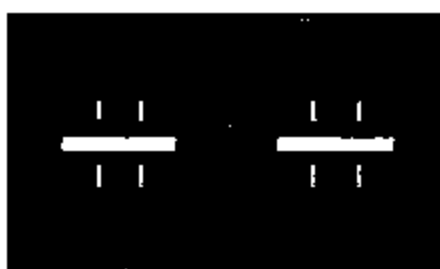
Routed Cut Line Relieves Stress on MLC
