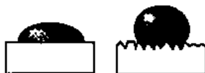
Fig. 3. Illustration of water contact angle for mirror surface and roughening surface. (a) For mirror surface, (b) for roughening surface.
