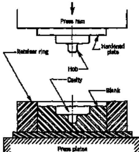
Figure 13.16 Die hob producing a mold cavity by pressing into soft steel.
