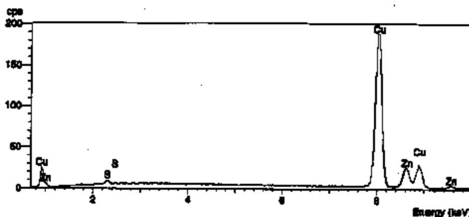
Figure 1: EDS X-ray spectrum of material scraped from the side of the stationary contact body.
