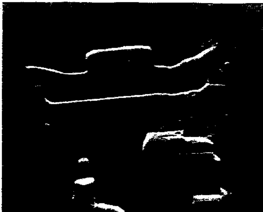
Figure 21: Fluorescopic image showing cracks and loss of material in stationary contact.
