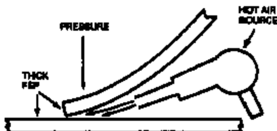
Illustration A. Hot Air Sealing of Thick Films
