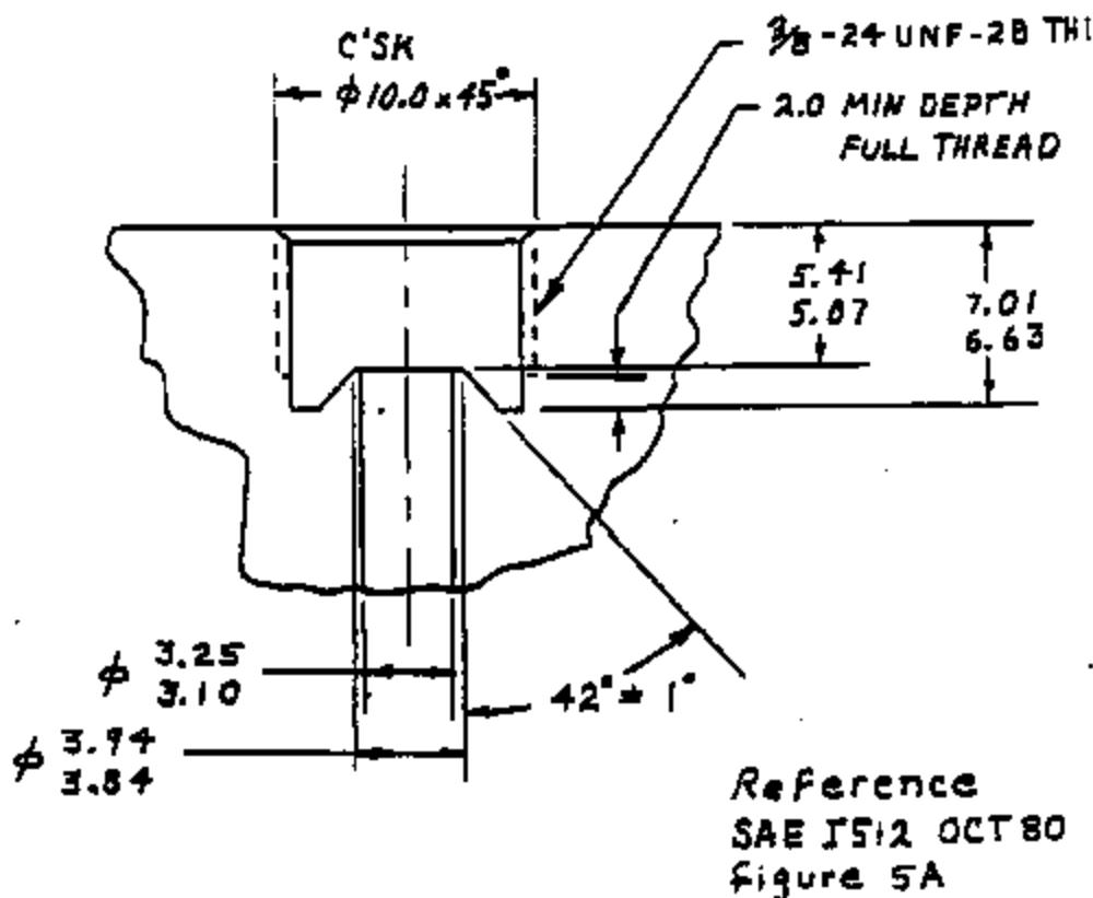
**TEST FIXTURE PORT CONFIGURATION**
