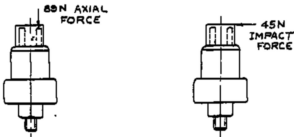
TERMINAL STRENGTH - LOAD ORIENTATION
