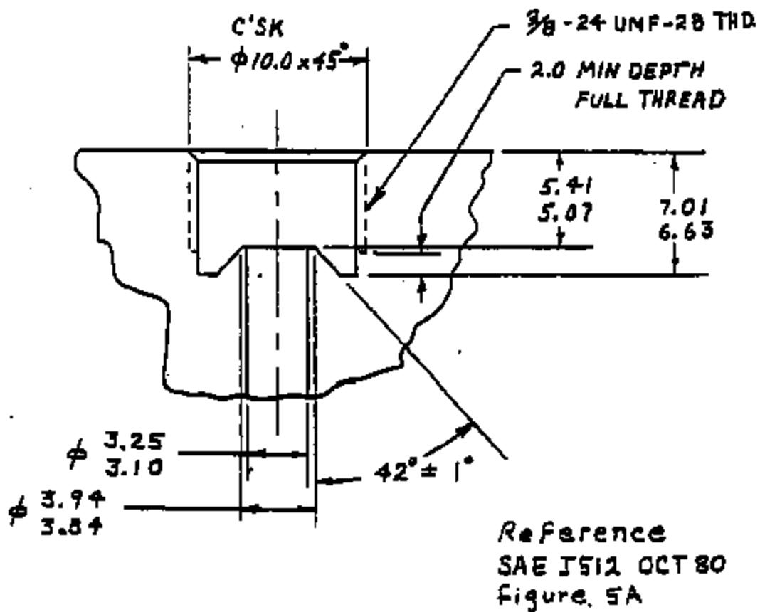
**TEST FIXTURE PORT CONFIGURATION**
