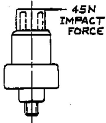
**TERMINAL STRENGTH - LOAD ORIENTATION**
