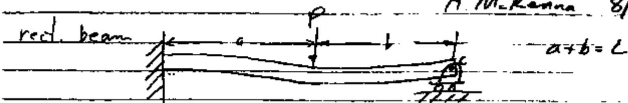
\* Calculate reaction force,  $P_c$ , at C for given load P:
