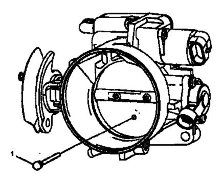
6. Insert the appropriate plug (1) into the sir bypass hole in the throttle plate. Insert the "tail" and of the plug through the throttle plate air bypass hole.
