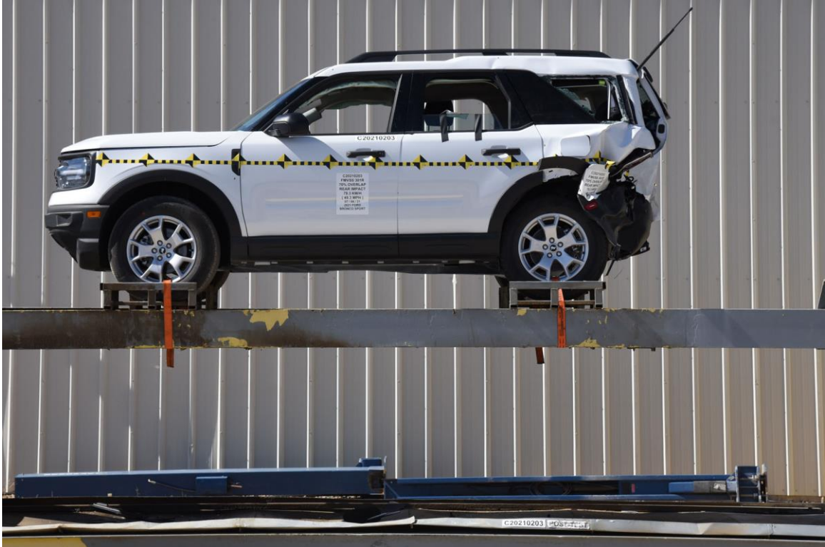
FIGURE 27. Test Vehicle at 36° on FMVSS 301 Static Rollover Device
