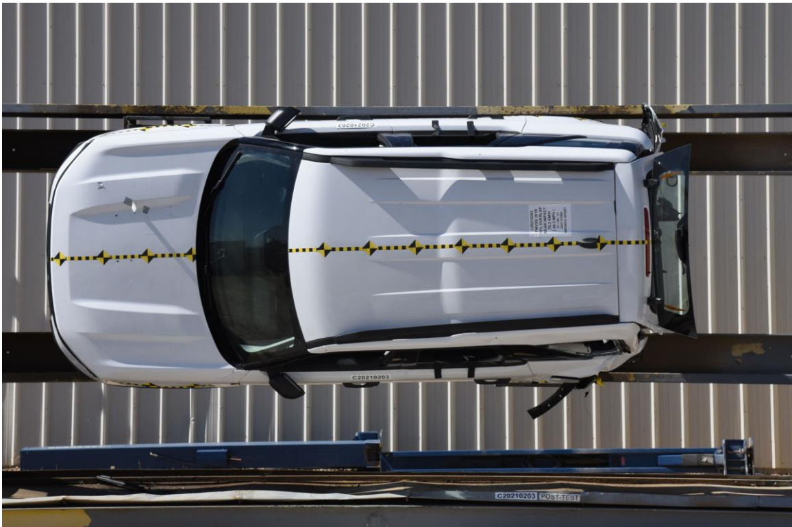
FIGURE 24. Test Vehicle at 90° on FMVSS 301 Static Rollover Device
