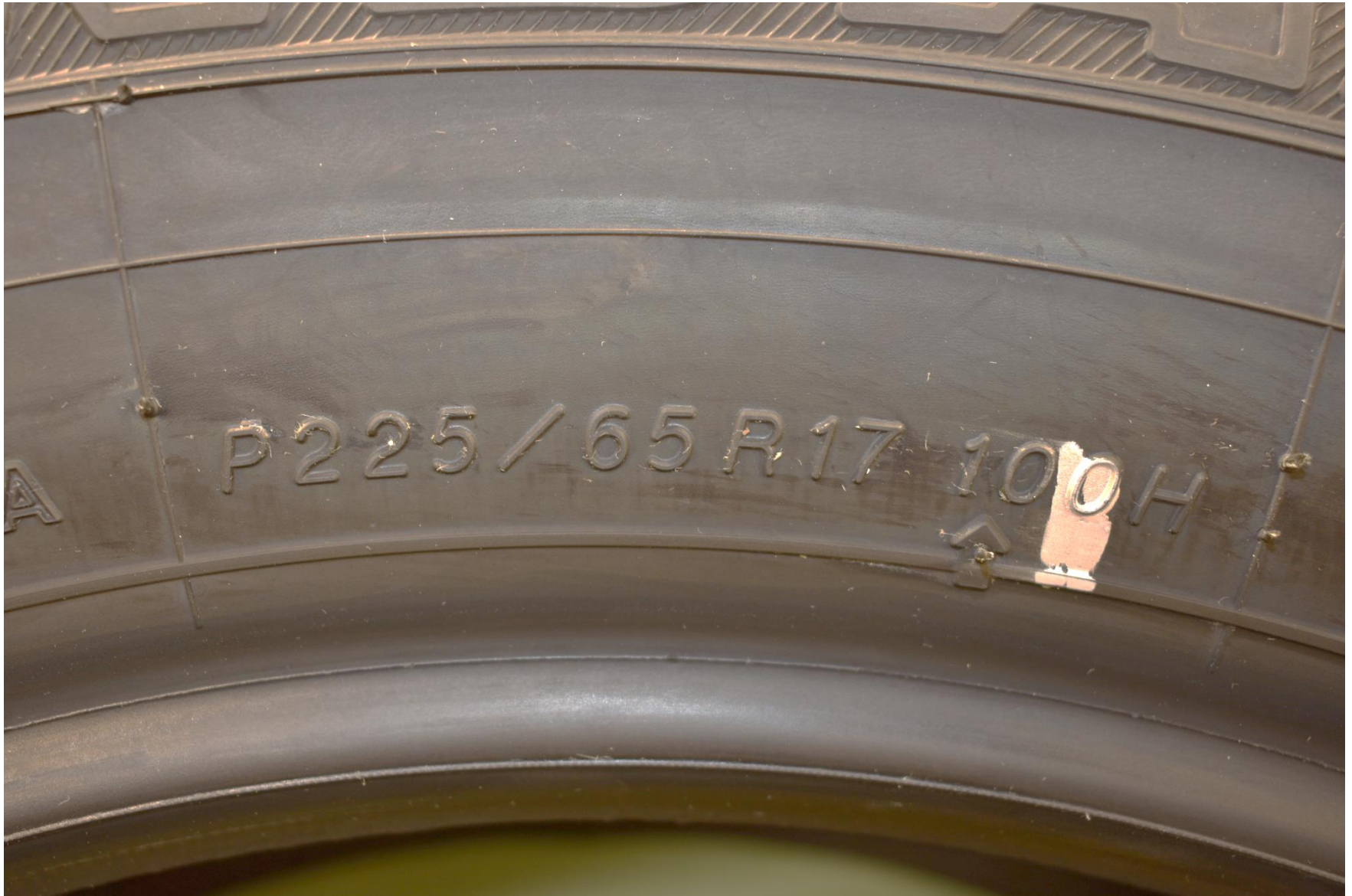
FIGURE 5.8 TIRE SHOWING SIZE, LOAD INDEX, AND SPEED SYMBOL
