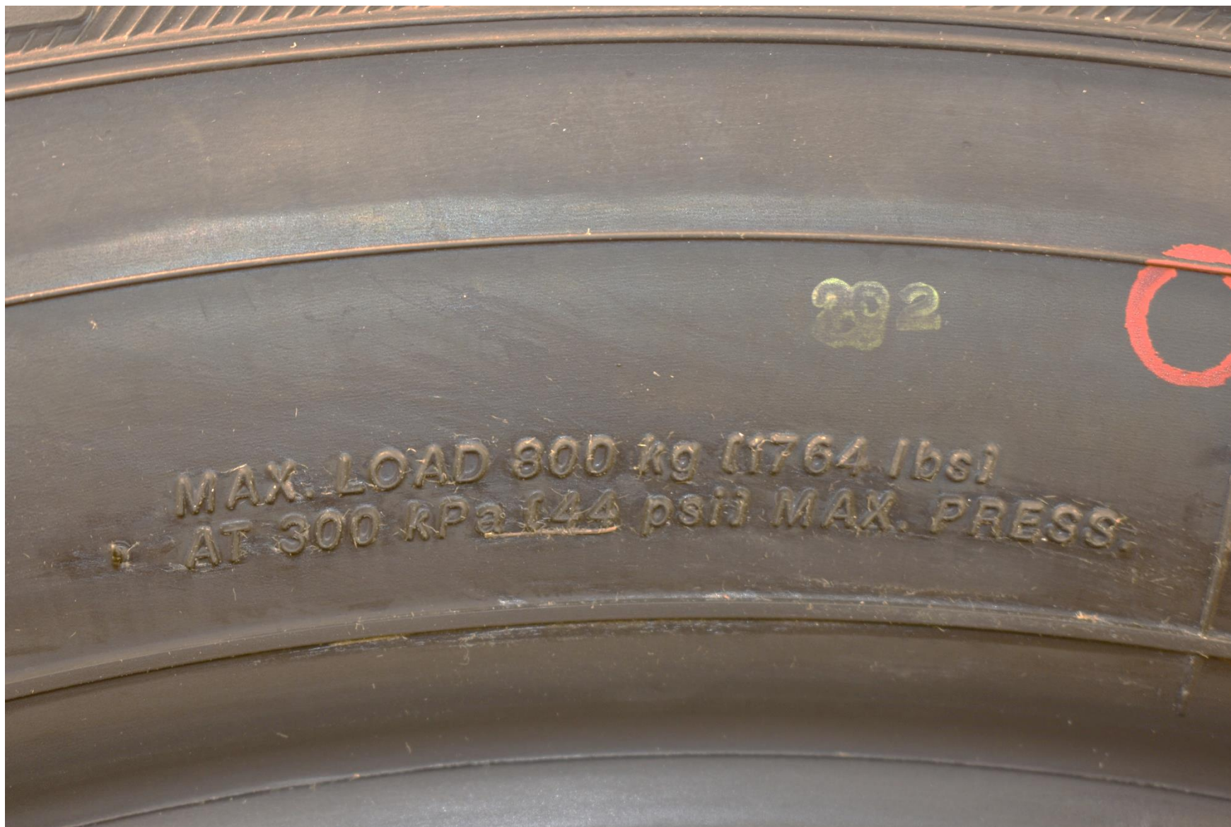
FIGURE 5.9 TIRE SHOWING MAX LOAD RATING AND MAX INFLATION PRESSURE
