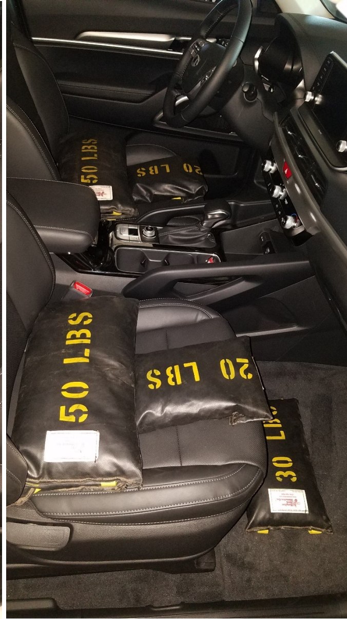
FIGURE 5.13 VEHICLE FRONT DRIVER AND PASSENGER SEATS BALLASTED FOR NORMAL, FULL, AND MAXIMUM LOADS
