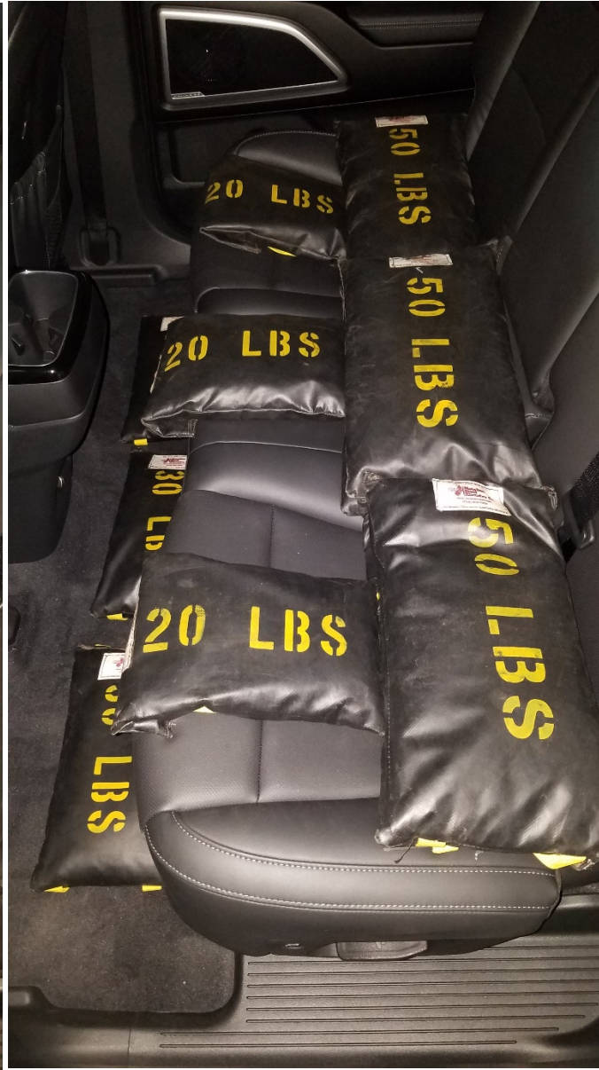
FIGURE 5.14 VEHICLE MID SEATS BALLASTED FOR NORMAL, FULL, AND MAXIMUM LOADS
