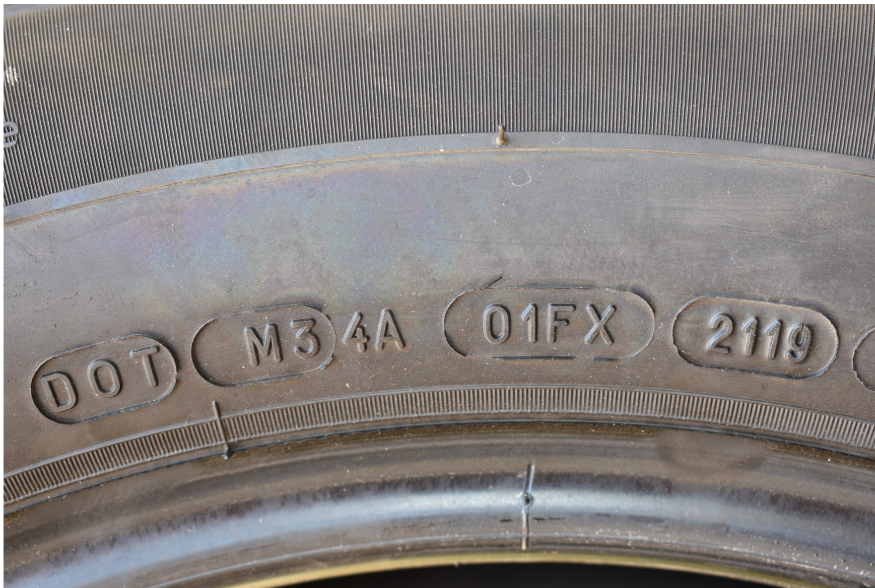
FIGURE 5.10 TIRE SHOWING SERIAL NUMBER
