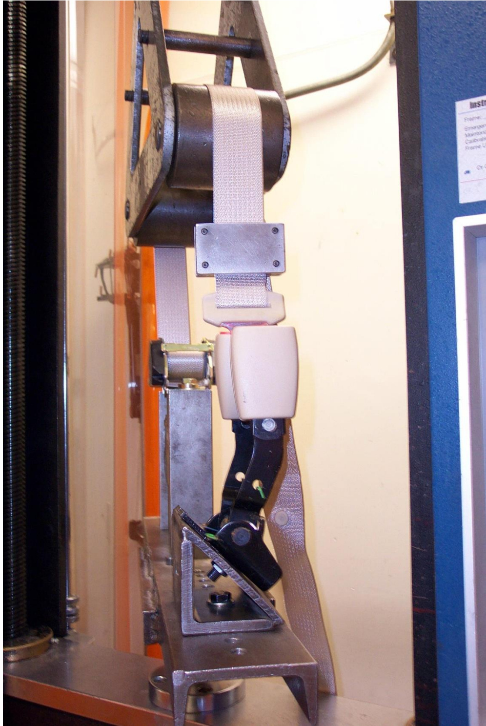
Loop Load Test
